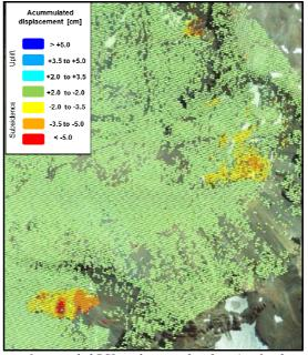
Figure 6: geocoded PSI total accumulated motion for the total time period.
