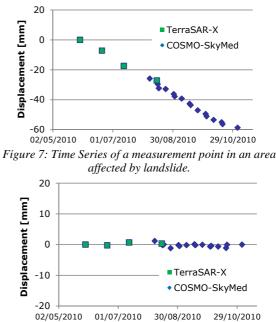
Figure 8: Time Series of a measurement point in a stable area.
