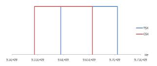
Figure 1: Range spectrums overlap between CSK and TSX SAR data in case of zero baseline and flat terrain.
