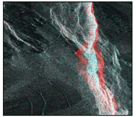
Figure 5: RGB image to show coregistration quality. Green and blue channels represent the CSK master amplitude, Red channel contains one TSX image in CSK geometry.
