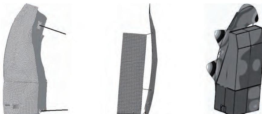
Figure 5.29. Structural analysis graphical results – thermoelastic distortion (left), lateral mode-shape (centre), axial mode shape (right) – deformations shown are exaggerated by orders of magnitude.
