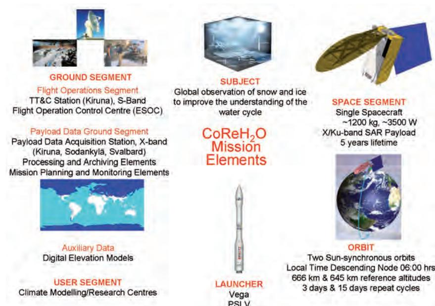
Figure 5.1. CoReH<sub>2</sub>O mission and system architecture.
