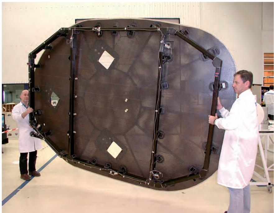
Figure 5.13. Astra-1K CFRP reflector (3.5 m x 2.6 m). (Astrium)
