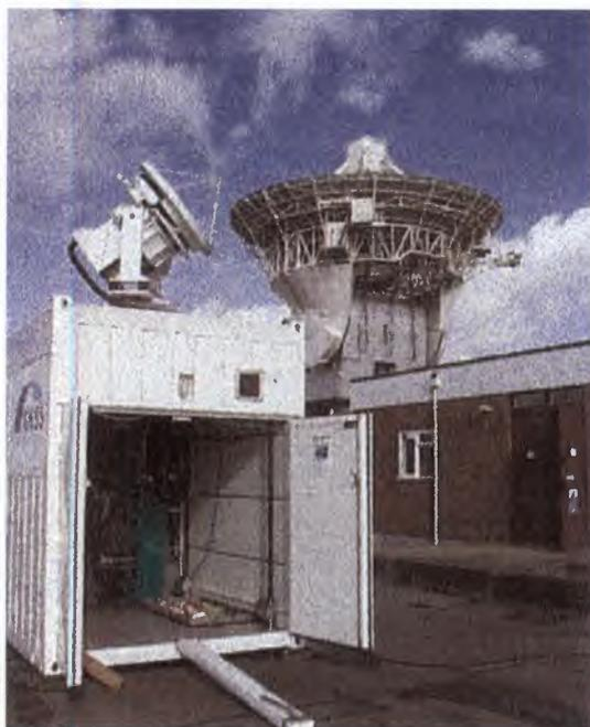
Fig. 1: The GKSS 95 GHz radar MIRACLE in front of the 3 GHz radar CAMRa during the campaign.
