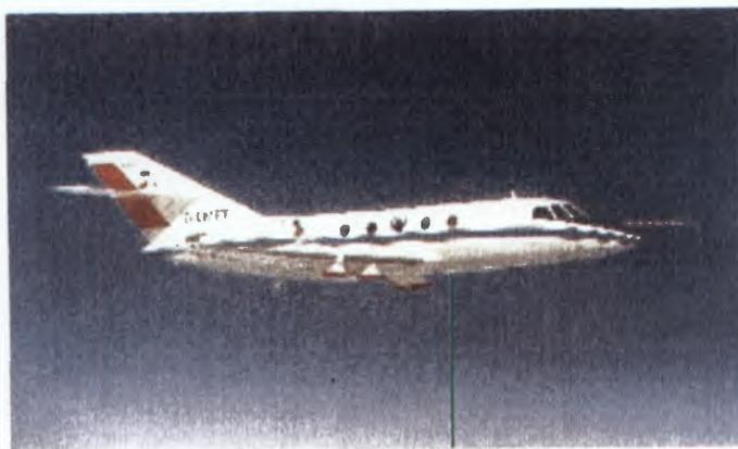
**Figure 1:** FALCON 20-E5 jet aircraft with lidar beam in downward-looking mode
