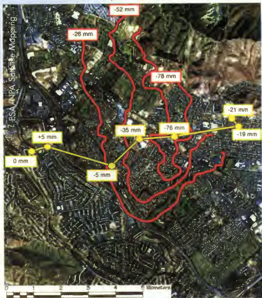
ERS SAR imagery is an important source of data for interferometric applications. This example shows how SAR imagery can be used to detect and measure subsidence in urban areas
