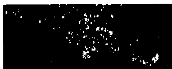
Fig. 5: A map corresponding to the detail image (Fig. 3) indicating where high dynamic data are located (high dynamic =1 (white), low dynamic =0 (black)) in the LH subband.
