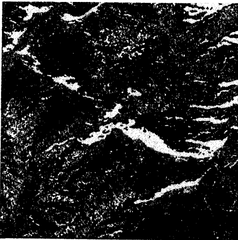
Fig. 7: C band, Izoard. Classified image using the direct Wishart classifier applied on 6 by 6 coherency matrices built from both April and October images.
