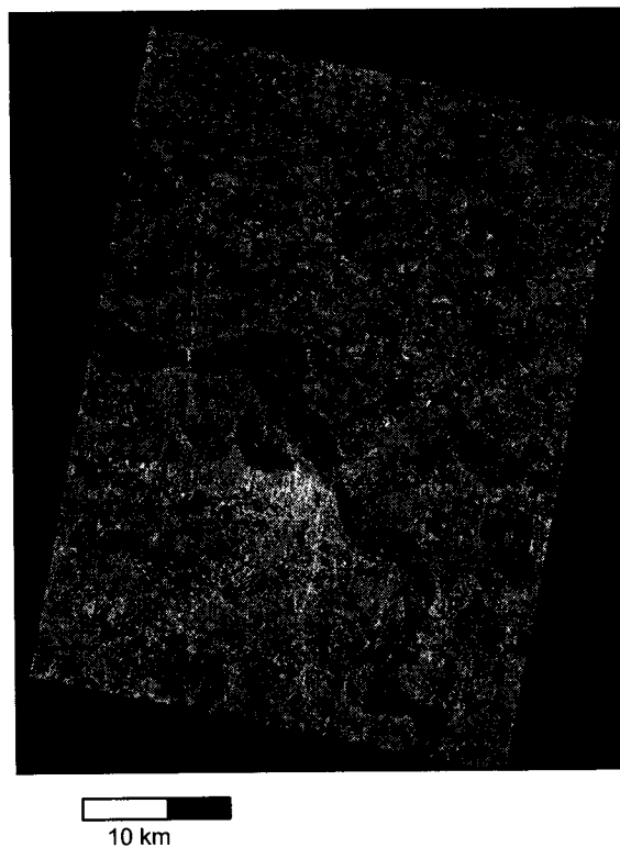
Fig. 3 : ERS SAR image registered to the SPOT image geometry
