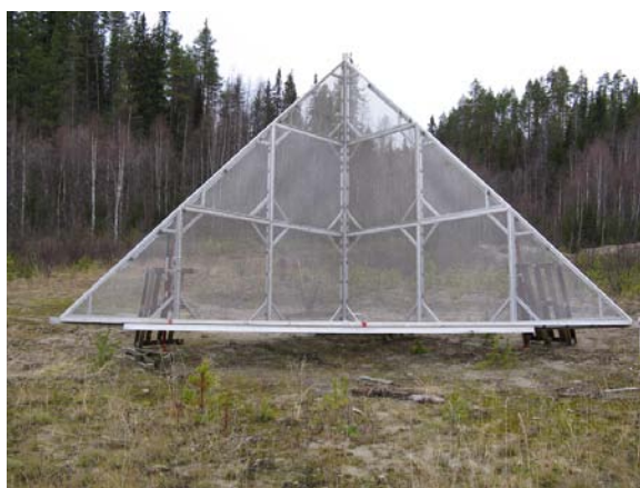
One of the large reflectors, CR2, could rest on the two available lift jacks instead of a wooden structure.
