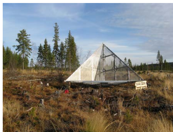
The required elevation for the large reflectors was adjusted using two lift jacks in each corner and then the trihedral rested on wooden structures, here CR4.
