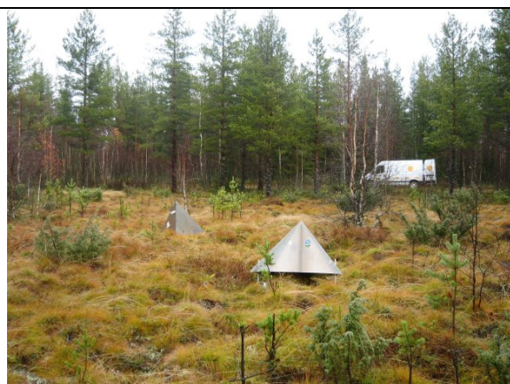
Corner Reflectors CR5A and CR5B (90cm)
