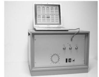
Figure 1: GOLD-RTR, IECC's GNSS-R hardware Receiver.
