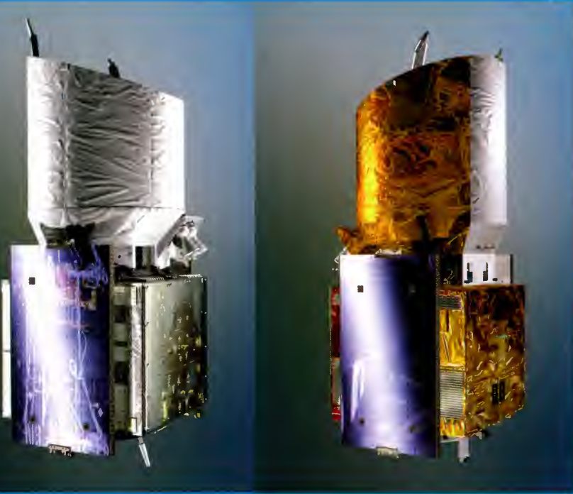
The Aeolus satellite in launch configuration with the solar arrays folded up. In the flight direction, the satellite has white covers that protect it from atomic oxygen erosion (left image), while the opposite sides of the satellite are covered with gold-coloured insulation for thermal control (right image).
