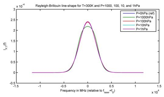
Figure 1: Rayleigh-Brillouin line-shapes for T=300K and different pressures P. The blue line is the classical Gaussian line-shape which serves here as a reference. The line-shapes for P=1hPa, 10hPa, 100hPa and 1000hPa are computed using Tenti S6 model. It can be seen that the departure from the Gaussian curve is larger as the pressure increases. The unit of the x-axis is MHz. The y-axis shows  $I_{PT}(f)$  in  $MHz^{-1}$ .
