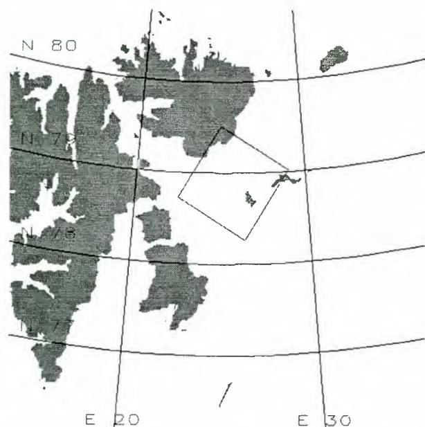
**Figure 1.** Data coverage at Kong Karls Land, east of Spitsbergen, Svalbard, for time series of ERS-1 synthetic aperture radar (SAR) images every 3 days at 1051 UTC January–March 1994 (given by the  $100 \times 100 \text{ km}^2$  frame).
