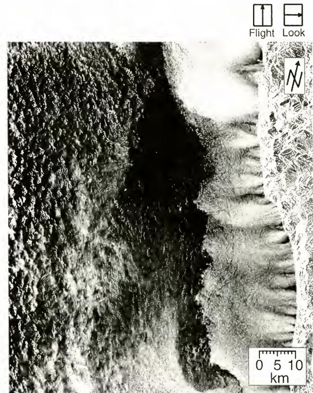
**Figure 2.** ERS-1 SAR image acquired on February 20, 1995, at 2113 UTC showing a sea surface roughness band stretching along the western Calabrian coast.
