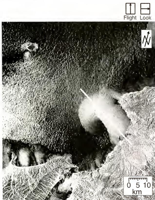
**Figure 3.** ERS-1 SAR image acquired on September 8, 1992, at 2114 UTC showing a “mushroom-like” roughness pattern in the Gulf of Gioia.
