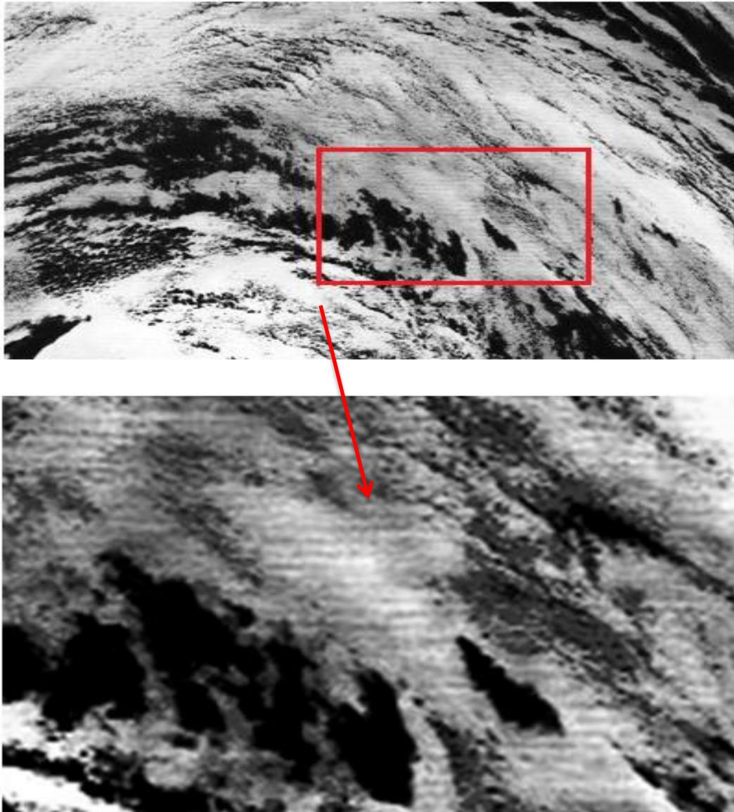
**Figure 1. An example of pick-up noise affecting measurements. Striations can be seen in the lower image, a close-up of the red boxed section of the upper image.**
