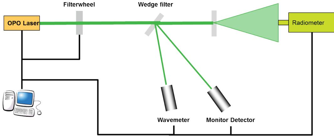
The Spectroradiometer entrance optic is placed in the center of the homogeneous radiation field produced by the microlens array, at a distance of about 20 cm to 30 cm. To select the best position, it is best to turn on the laser, set it a visible wavelength, e.g. 550 nm, and adjust the entrance optic of the Device Under Test (DUT) until it is fully illuminated.
