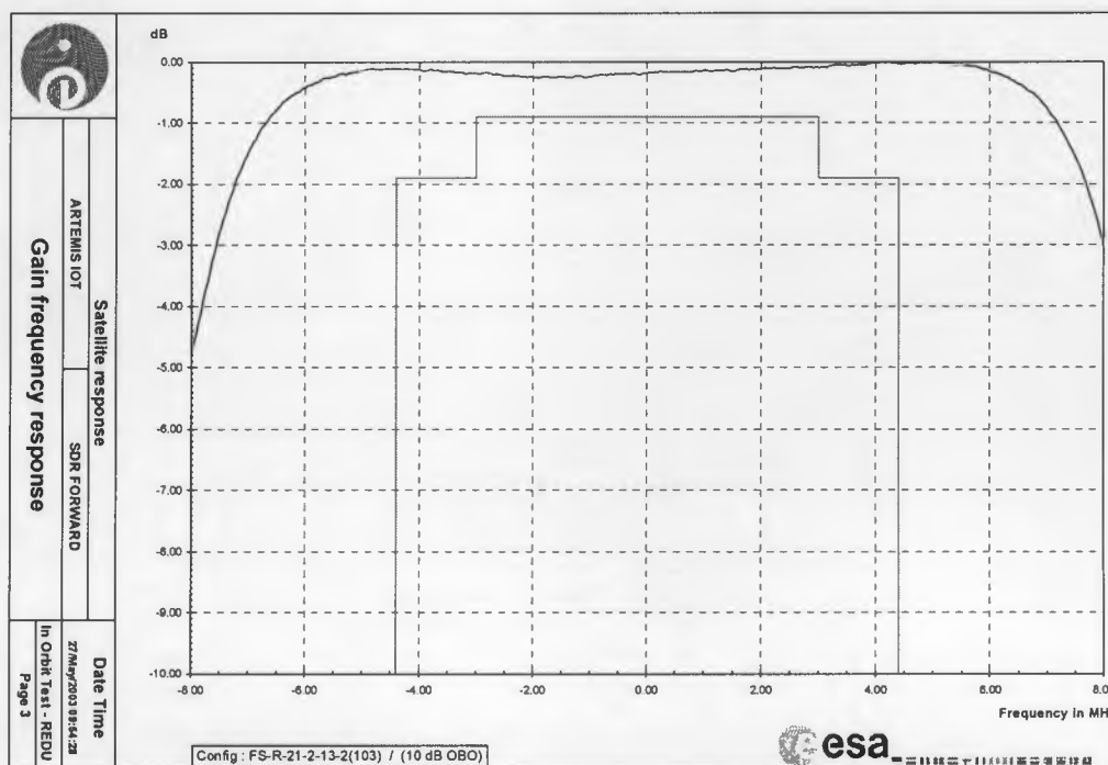
Figure 26 30/2 GHz channel (S-FWD) gain / frequency response
