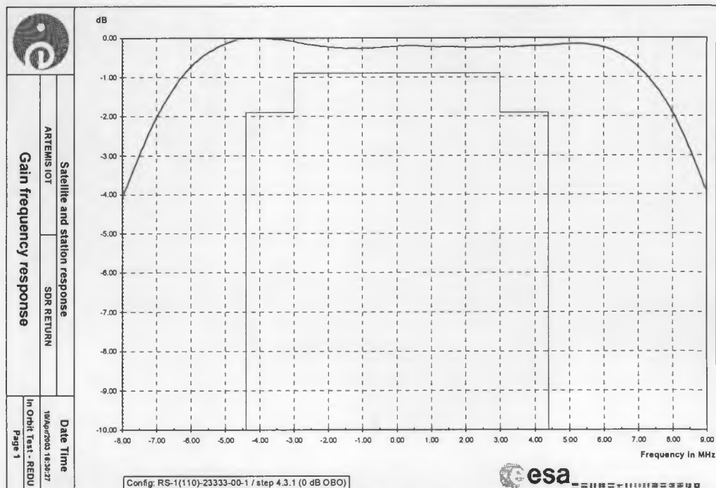
Figure 28 20 / 2.2 GHz channel gain/frequency response
