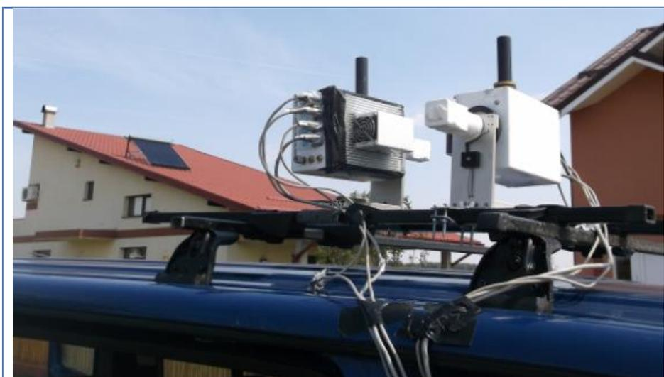
Figure 10: Two Mini-MAX-DOAS instruments mounted on the roof of the car.
