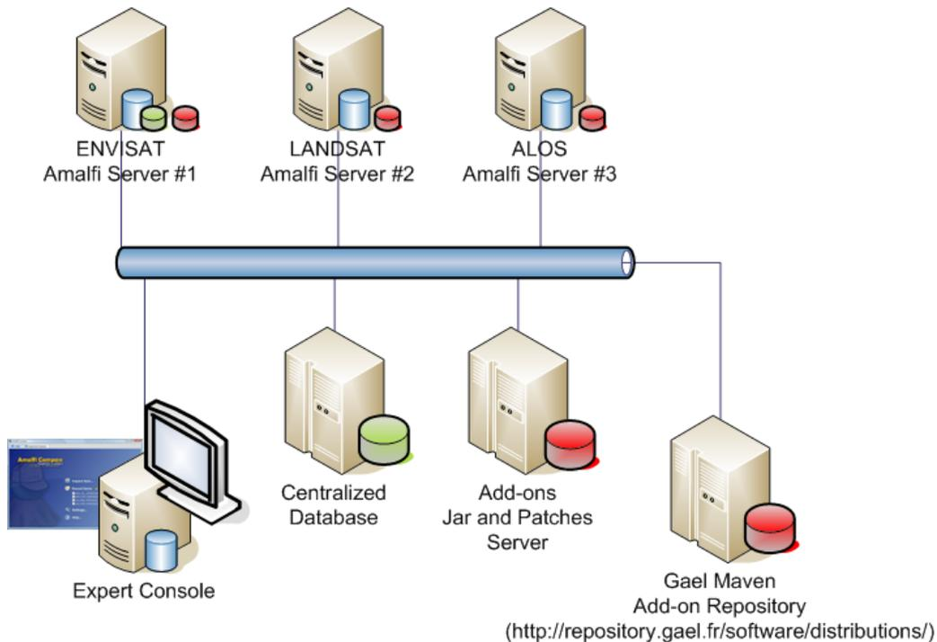
fig. 39 - Amalfi physical deployment sample
