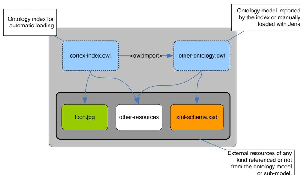
fig. 36 - Anatomy of a typical Add-on of DRB Cortex extension
