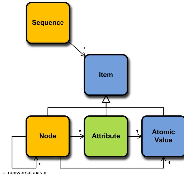
fig. 40 - Amalfi static data model
