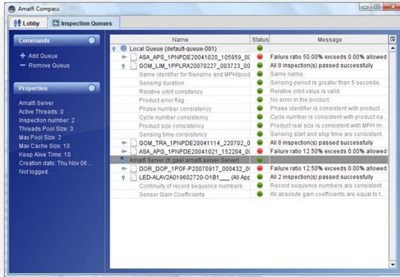
fig. 22 - Amalfi Compass - Multiple inspection queues
