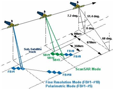
Figure 1: The 132 PALSAR observation modes, resulting from the combination of 18 different off-nadir beams for strip SAR and five observation modes (FBS, FBD, FL, SL, P)
