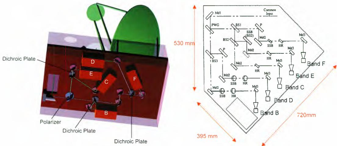
**Figure 6.5:** Two possible MASTER quasi optical designs (left – layout I, right – layout II, for right panel: PWG = polarising wire grid, BS = beam splitter, SSB = single sideband filter, HR = harmonic rejection filter, P = planar mirror, Md1 and Md2 = ellipsoidal mirror and Md3 = redundancy switching mirror).
