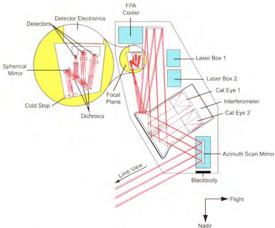
**Figure 6.7:** AMIPAS overall optical configuration.
