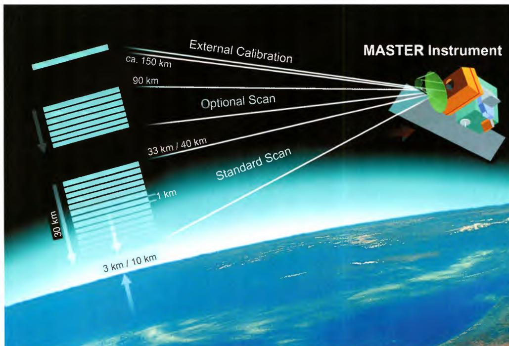
**Figure 6.2:** MASTER observation geometry, showing the standard scan range and the extended scan ranges achieved by the platform.
