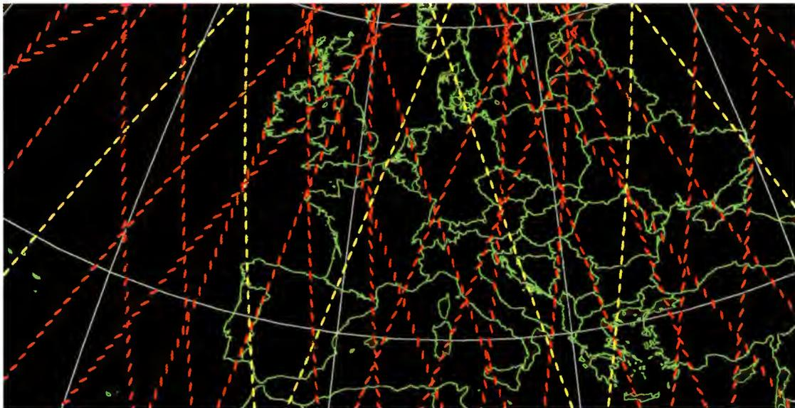
*Figure 6.17: European coverage of limb sounders in a 24 h period: the yellow marks represent the MASTER scans and the central AMIPAS measurement; the red marks indicate the azimuth views of AMIPAS.*
