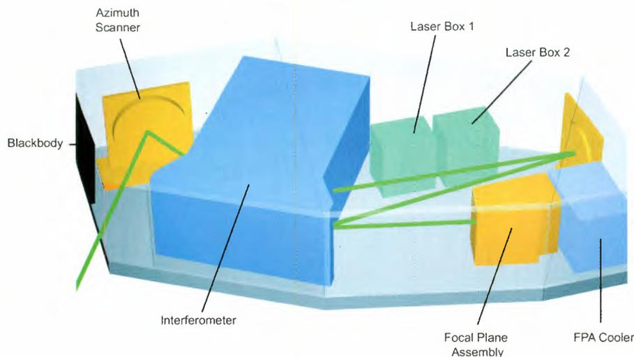
**Figure 6.8:** Optics Module optomechanical configuration.
