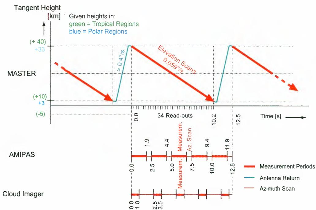
Figure 6.1a: Scanning scheme for all ACECHEM instruments, showing the temporal interleaving of the scans of the different instruments.
