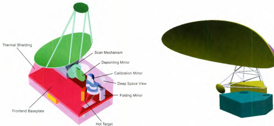
**Figure 6.6:** The MASTER instrument in two envisaged configurations.
