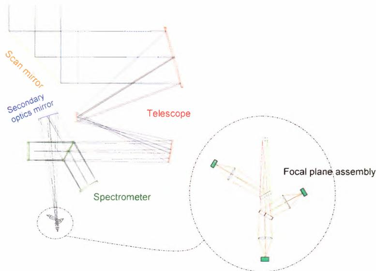
**Figure 6.9:** Concept II optical layout.
