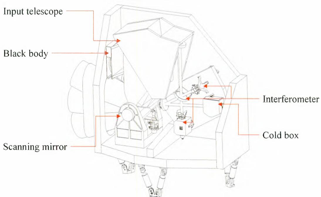
**Figure 6.10:** Overall mechanical layout.
