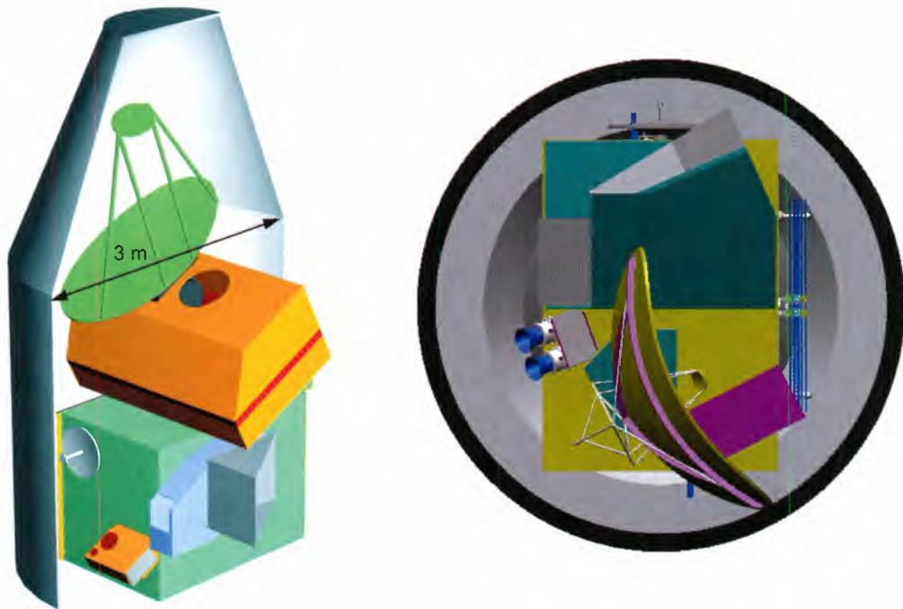
**Figure 6.19:** ACECHEM Configuration I (left) and Configuration II (right) in stowed configuration in the Soyuz launcher.
