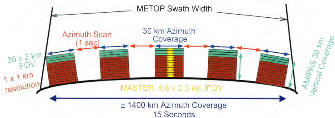
Figure 6.1b: Limb view of ACECHEM satellite: The green grid (partially hidden) represents the AMIPAS acquisition. The red grid corresponds to the Cloud Imager, and the yellow ellipses indicates the collocation of the MASTER field of view for the along-track direction. The red lines indicate the MetOp swath (drawing not to scale).
