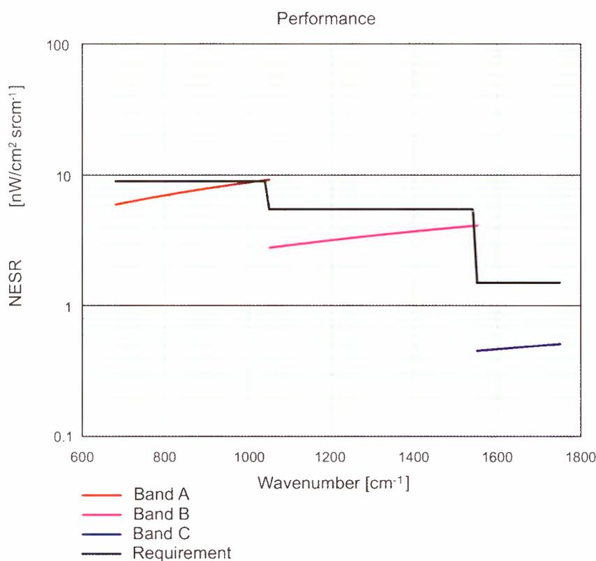
**Figure 6.11:** Simulated NESR versus wavenumber for an instrument optics temperature of 160 K.
