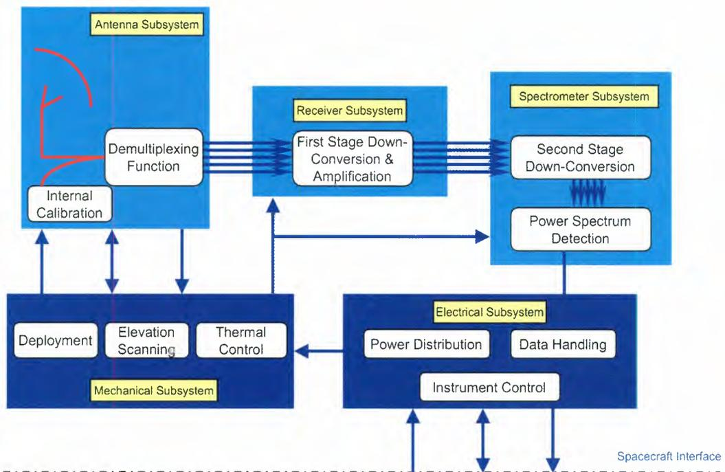
**Figure 6.3:** MASTER functional block diagram.
