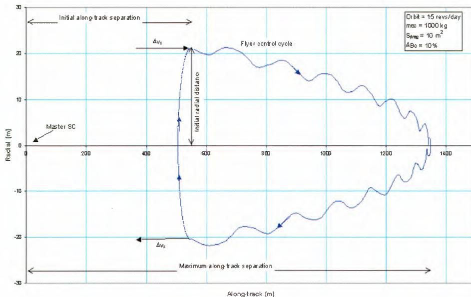
**Figure 6.16:** Control cycle with differential ballistic coefficient.
