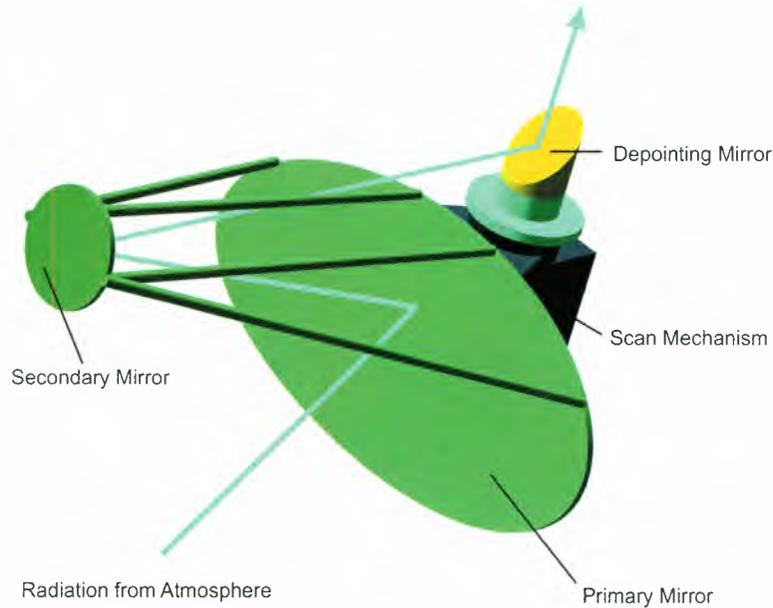
**Figure 6.4:** The MASTER antenna system, illustrating the beam path.
