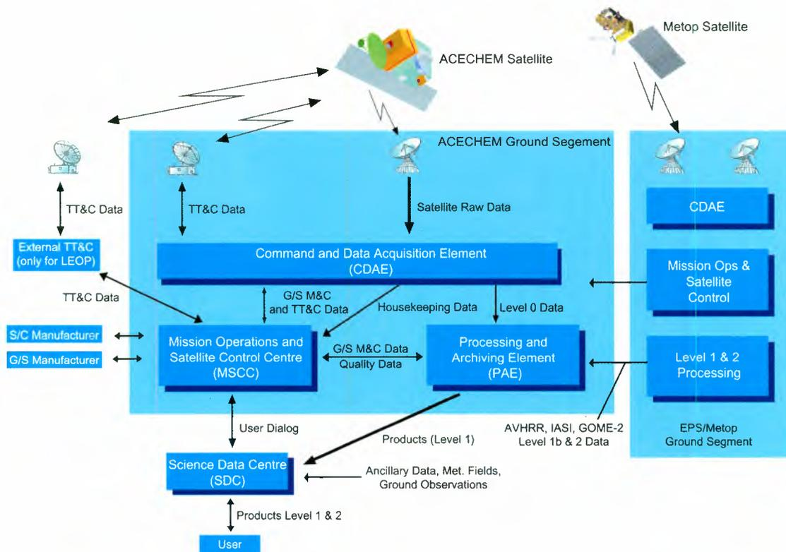
*Figure 6.18: ACECHEM Ground Segment reference architecture.*
