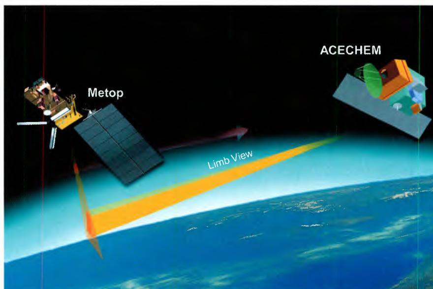
*Figure 5.1: Overall observation geometry of the ACECHEM mission.*
