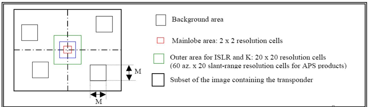
**Figure 1** Definition of point target response area and background areas for IRF analysis and calibration.
