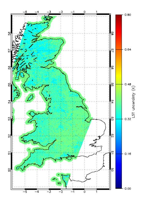
Figure 4: Example for the LST uncertainty derived from (A)ATSR
