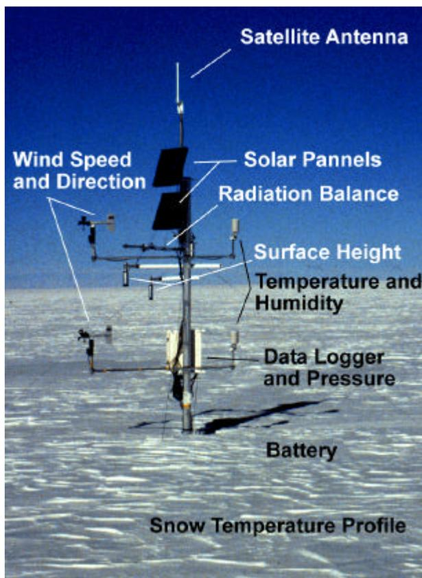
Figure 11.4.3.1-1 Automatic Weather Station situated in Greenland
