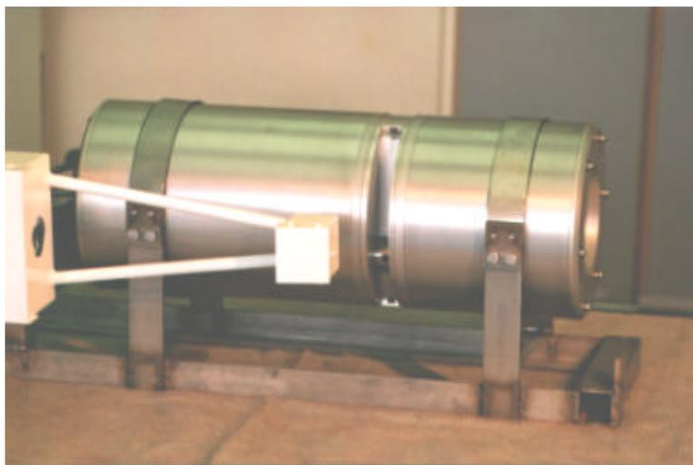
Figure 9.2.1.1-1 The Infrared Autonomous SST Radiometer (ISAR5C) shown together with the optical rain gauge in place. The rain gauge is used to control the opening/closing of a shutter system that seals the instrument from rain and sea spray during bad weather. The shutter is open in this picture revealing the small viewing aperture and scan drum assembly.
