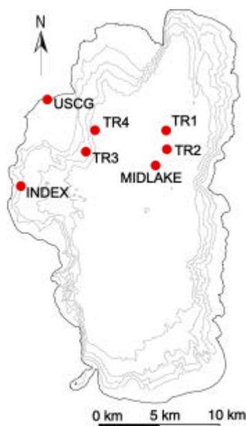
Figure 11.1.5.1-1. Bathymetric map of Lake Tahoe with a contour interval of 100 m. The 4 NASA rafts are labelled TR1, TR2, TR3 and TR4. Also shown is the US Coast Guard station (USCG), Midlake and Index stations. A variety of atmospheric measurements are made at the USC and a variety of water properties are measured at the Midlake and Index stations.
