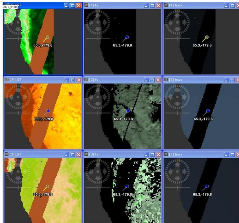
Figure 1. Three LST products (see Table 1) displaying an anomalous LST strip in the Bering peninsula. Left to right: LST, fractional vegetation cover (fv) and total column water vapour (tcwv).
