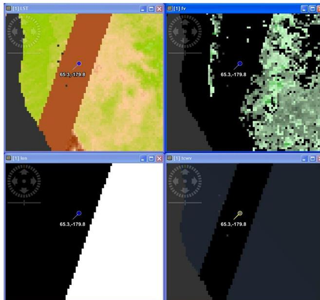
**Figure 4. The anomalous bands of product (3) shown with longitude (bottom left). The transition from black to white in the longitude band signals the 180<sup>th</sup> meridian.**
