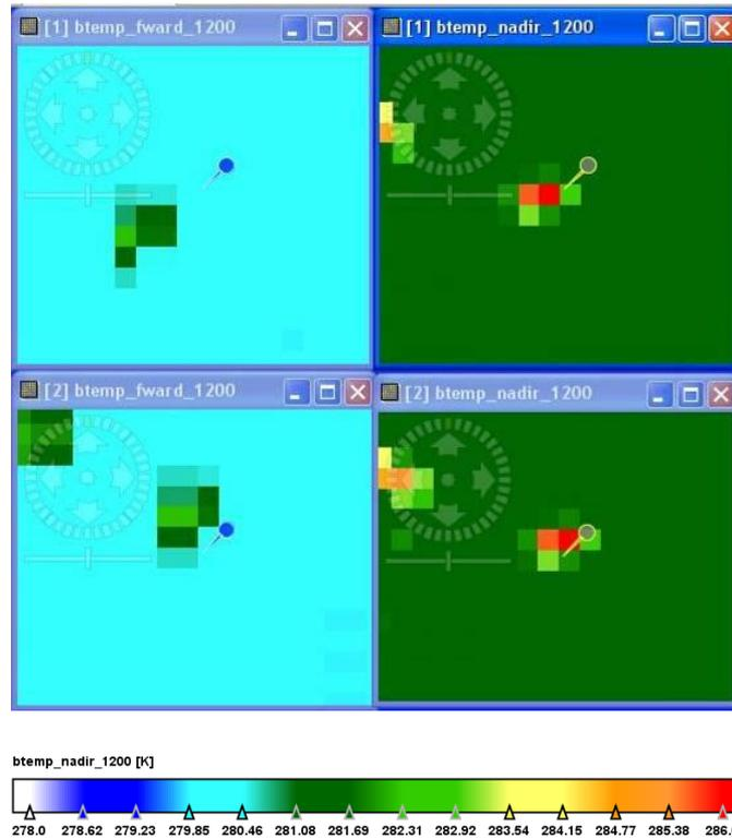
**Figure 4. BEAM image of the 12 μm brightness temperatures for the 2<sup>nd</sup> (top) and 3<sup>rd</sup> reprocessings (bottom) of AATSR for Hoedic. Left: forward view; right: nadir view. The pin is at the location of the island specified in Table 1.**
