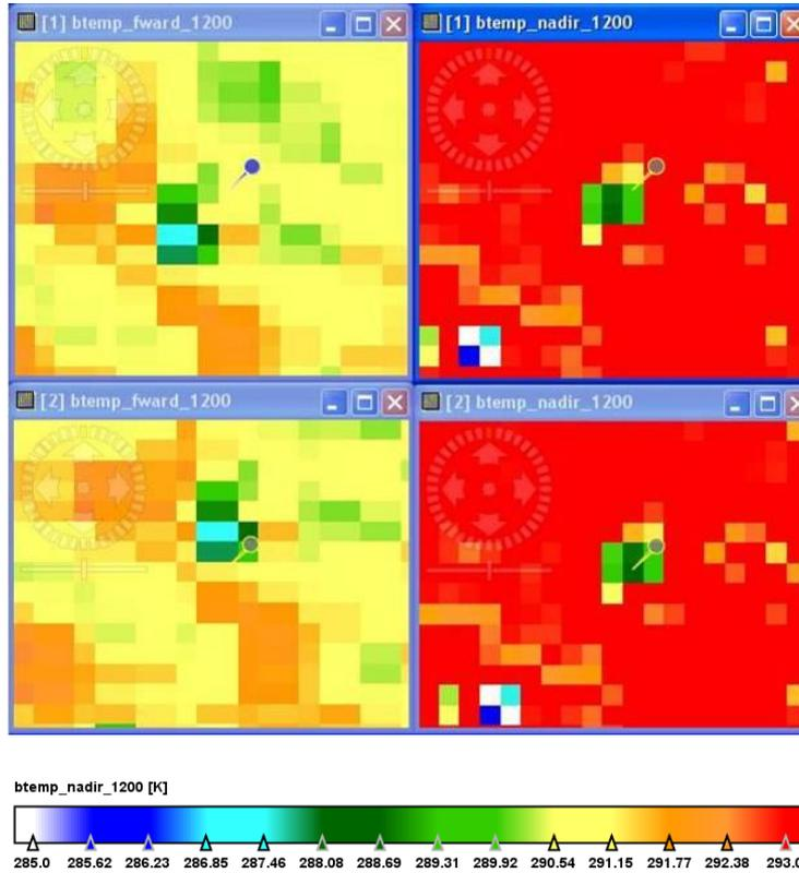
**Figure 6. BEAM image of the 12  $\mu$ m brightness temperatures for the 2<sup>nd</sup> (top) and 3<sup>rd</sup> reprocessings (bottom) of AATSR for Lake Otno. Left: forward view; right: nadir view. The pin is at the location of the lake specified in Table 1.**
