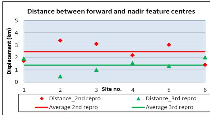
**Figure 10. Distance (km) between the weighted centres of the forward and nadir features for the 2<sup>nd</sup> and 3<sup>rd</sup> reprocessings.**
