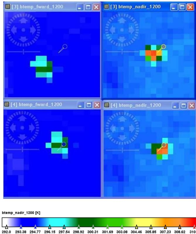
**Figure 3. BEAM image of the 12  $\mu$ m brightness temperatures for the 2<sup>nd</sup> (top) and 3<sup>rd</sup> reprocessings (bottom) of AATSR for Linosa, orbit 33198. Left: forward view; right: nadir view. The pin is at the location of the island specified in Table 1.**
