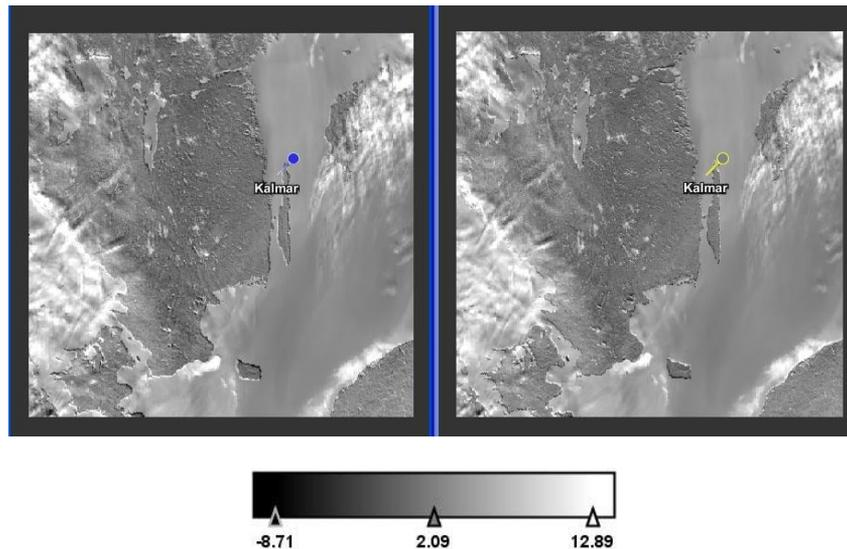
Figure 15. The forward–nadir difference image (0.87 μm) for 2<sup>nd</sup> reprocessing data (left) and 3<sup>rd</sup> reprocessing data (right) for a 512 x 512 pixel scene around the island in the Kalmar strait.
