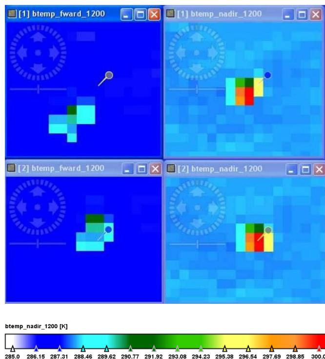
**Figure 2. BEAM image of the 12  $\mu\text{m}$  brightness temperatures for the 2<sup>nd</sup> (top) and 3<sup>rd</sup> reprocessings (bottom) of AATSR for Linosa, orbit 32468. Left: forward view; right: nadir view. The pin is at the location of the island specified in Table 1.**
