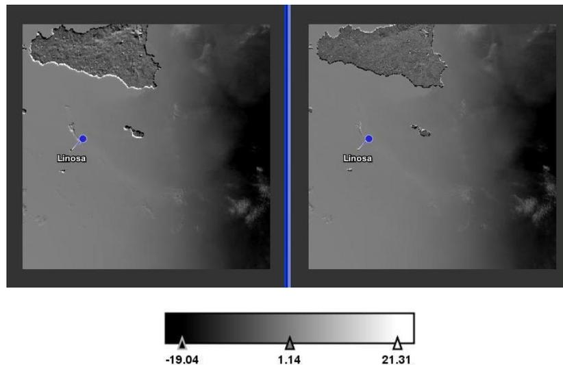
Figure 17. The forward-nadir difference image (0.87  $\mu\text{m}$ ) for 2<sup>nd</sup> reprocessing data (left) and 3<sup>rd</sup> reprocessing data (right) for a 512 x 512 pixel scene around Linosa (orbit 33198).
