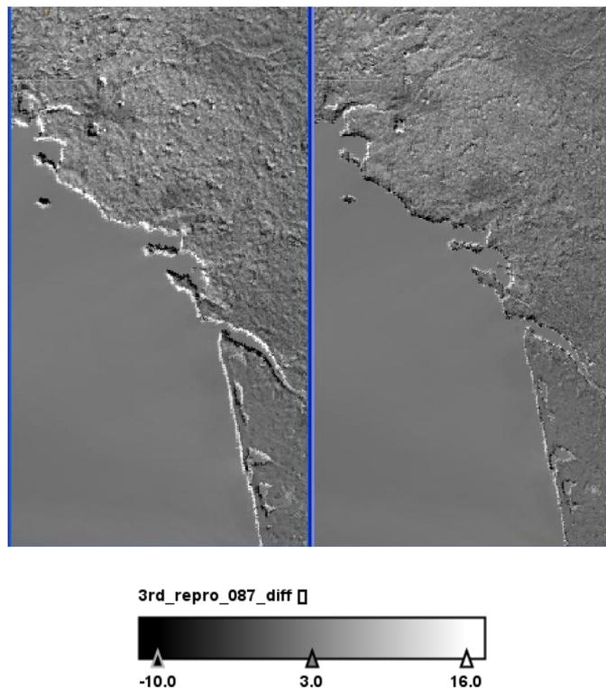
**Figure 21. The forward-nadir difference image (0.87  $\mu\text{m}$ ) for 2<sup>nd</sup> reprocessing data (left) and 3<sup>rd</sup> reprocessing data (right) from the Hoedic products.**
