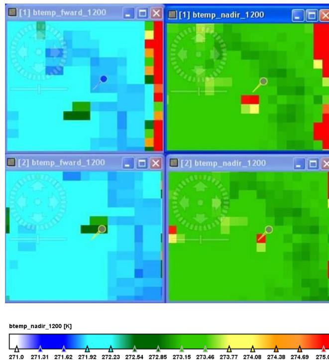
**Figure 1. BEAM image of the 12 μm brightness temperatures for the 2<sup>nd</sup> (top) and 3<sup>rd</sup> reprocessings (bottom) of AATSR for the island in Kalmar strait. Left: forward view; right: nadir view. The pin is at the location of the island specified in Table 1.**
