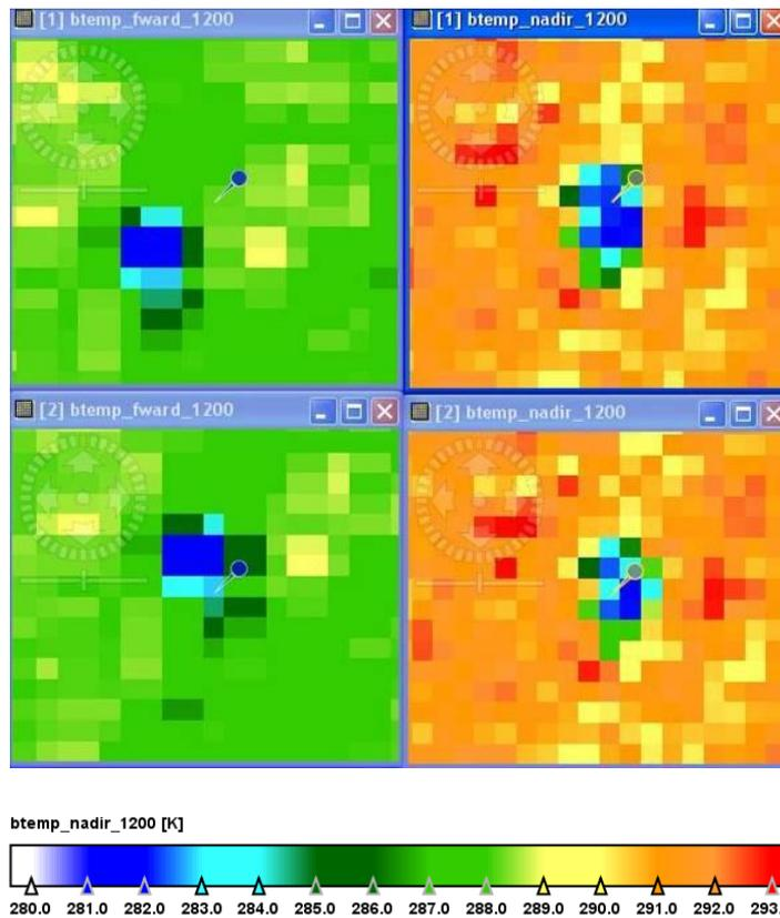
**Figure 5. BEAM image of the 12 μm brightness temperatures for the 2<sup>nd</sup> (top) and 3<sup>rd</sup> reprocessings (bottom) of AATSR for Lake Aluksne. Left: forward view; right: nadir view. The pin is at the location of the lake specified in Table 1.**
