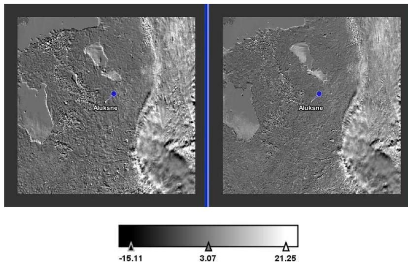
Figure 19. The forward–nadir difference image ( $0.87 \mu\text{m}$ ) for 2<sup>nd</sup> reprocessing data (left) and 3<sup>rd</sup> reprocessing data (right) for a 512 x 512 pixel scene around Lake Aluksne.
