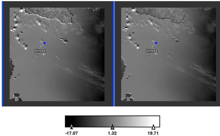
Figure 16. The forward-nadir difference image (0.87  $\mu\text{m}$ ) for 2<sup>nd</sup> reprocessing data (left) and 3<sup>rd</sup> reprocessing data (right) for a 512 x 512 pixel scene around Linosa (orbit 32468).
