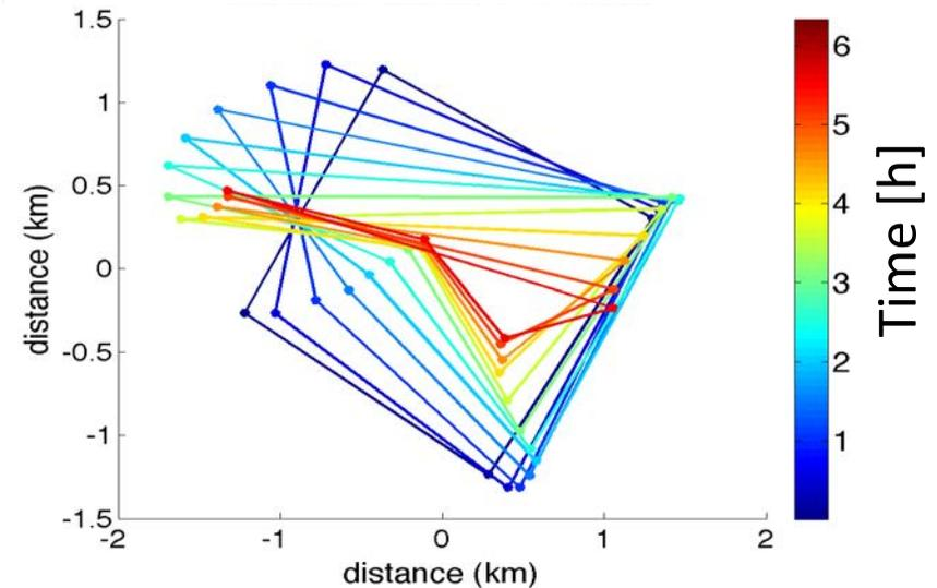
Relative motion within drifter clusters provide velocity differentials. Divergence and vorticity is quantified from differential kinematic property calculations.
