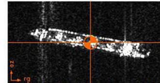
TerraSAR-X image, patch size (rg x az): 203 x 102 px. The circle marks the pixel considered for geocoding.
