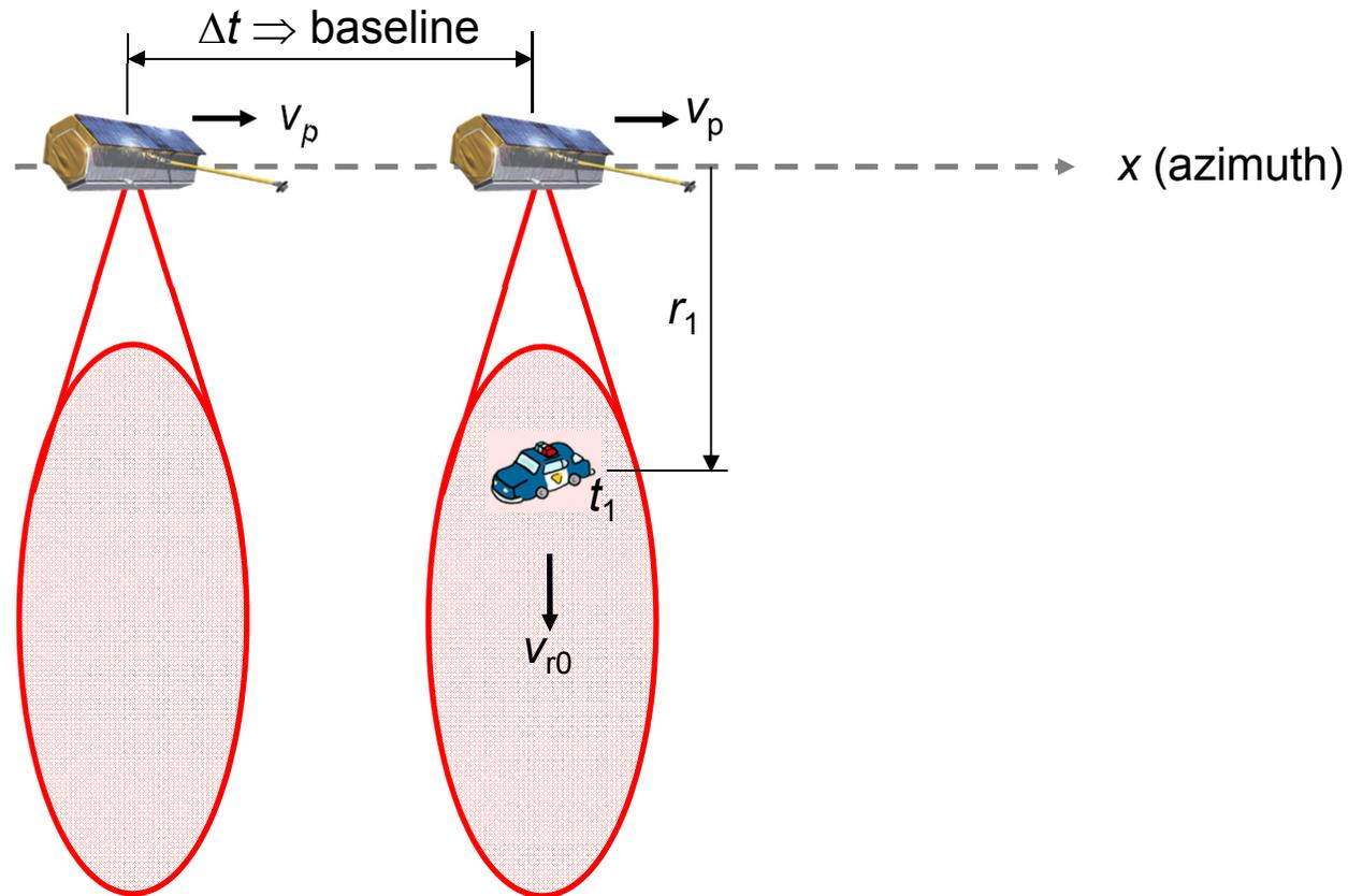
The RX antennas are separated in flight or along-track (azimuth) direction, respectively.
