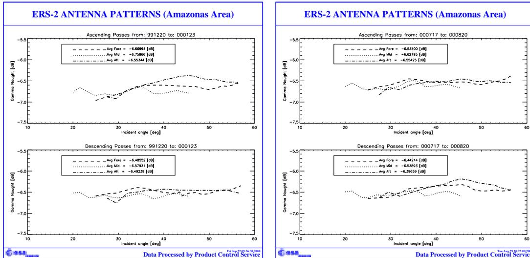
Fig. 2 ERS-2 WindScatterometer: Antenna Pattern profiles over the Rain Forest. Left panel winter profiles, right panel summer profiles
