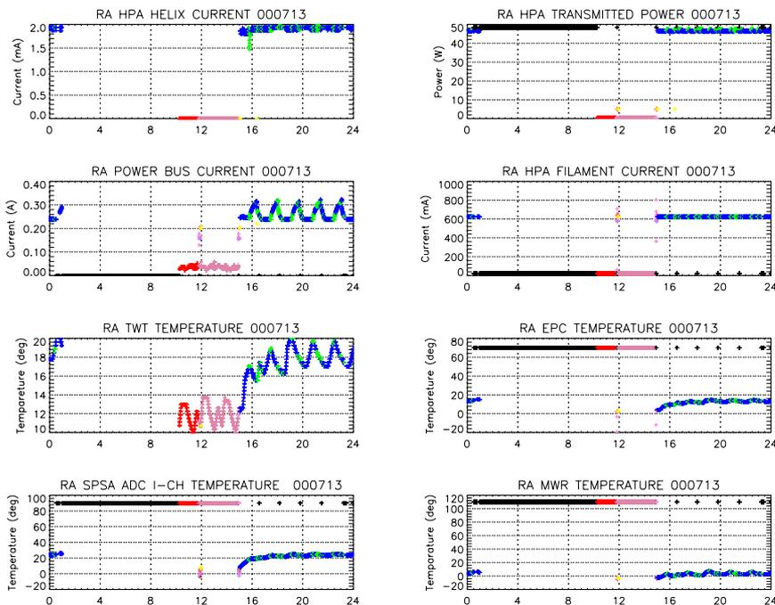
Fig. 8 ERS-2 RA internal parameters variations in occasion of an anomaly
