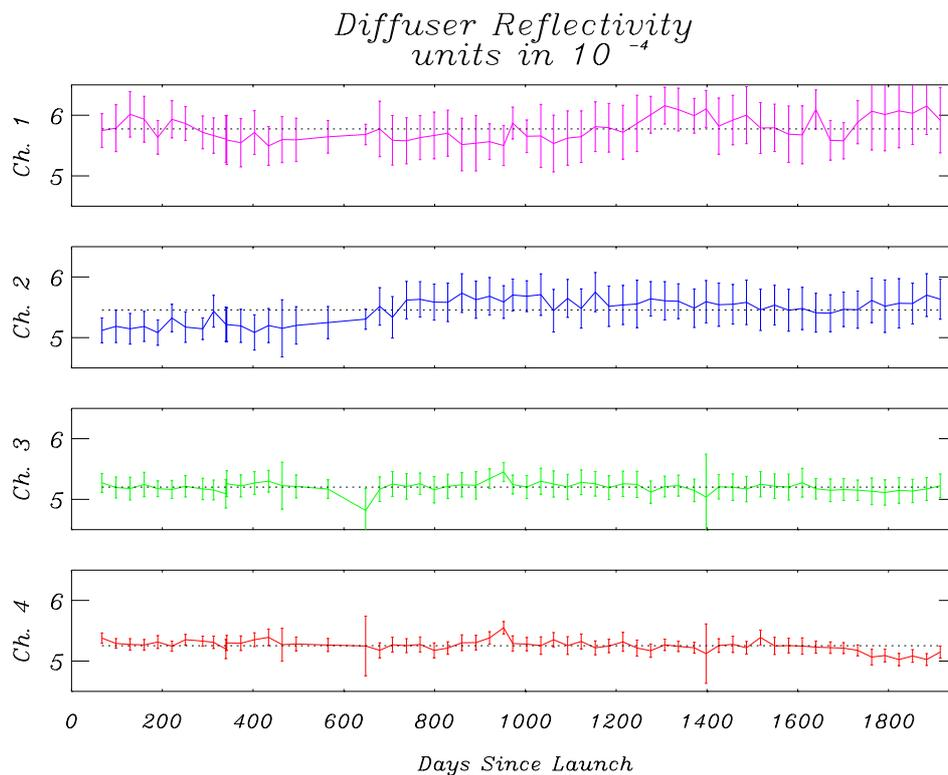
Fig. 6 GOME Diffuser Reflectivity (27/06/1995 – 28/07/2000)
