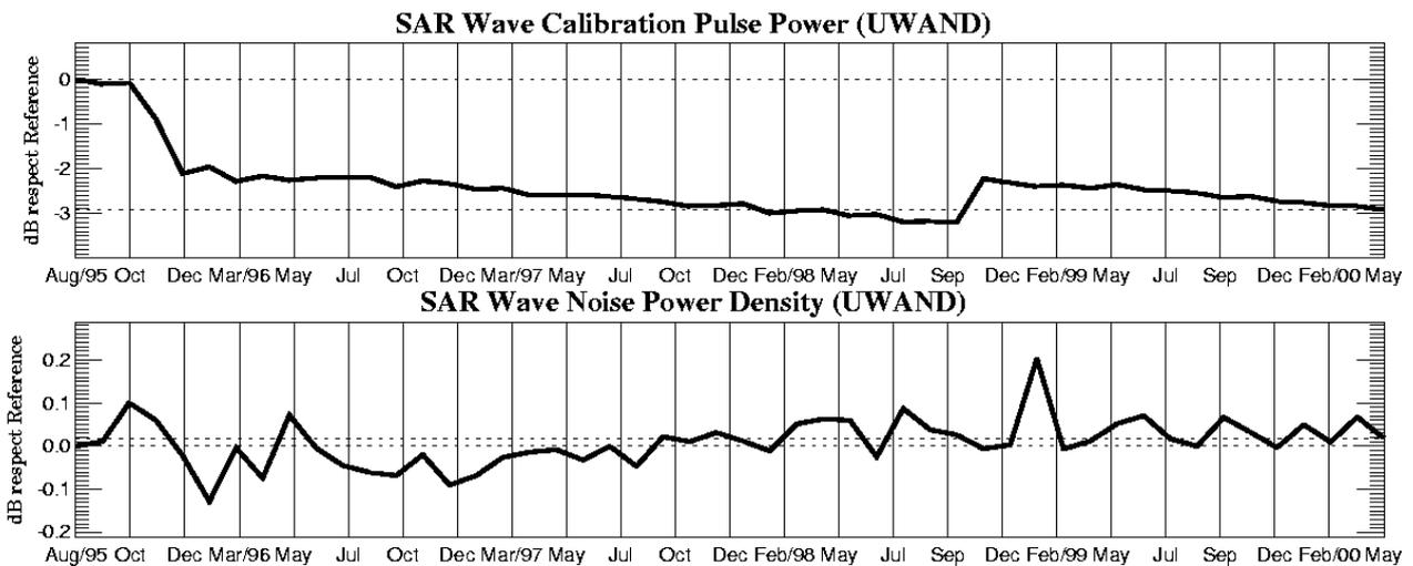
Fig. 12 ERS-2 SAR (Wave mode) Calibration power (upper plot) and Noise power (lower plot) evolution
