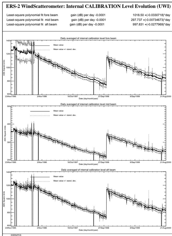
Fig. 10 ERS-2 WindScatterometer: Internal calibration evolution since the beginning of the mission.
