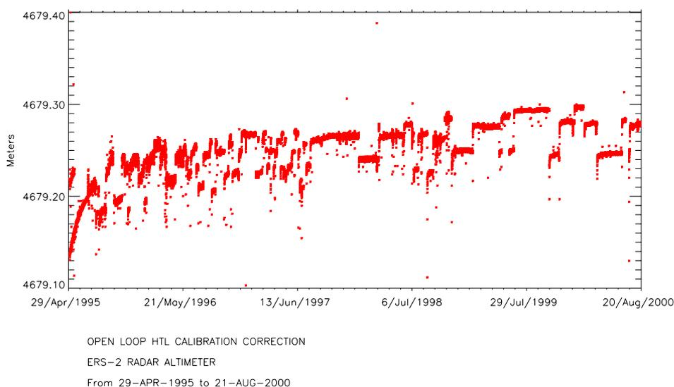
Fig. 4 ERS-2 RA Open Loop Height Tracking Loop Calibration Correction evolution over the whole mission
