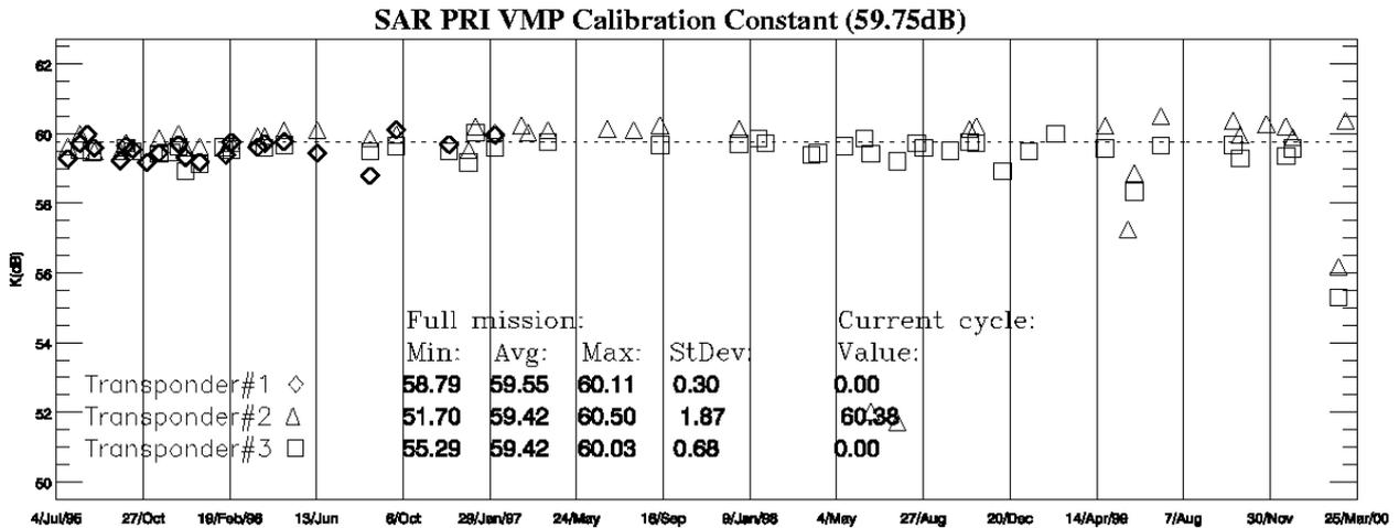
Fig. 11 ERS-2 SAR Calibration constants over Transponders.
