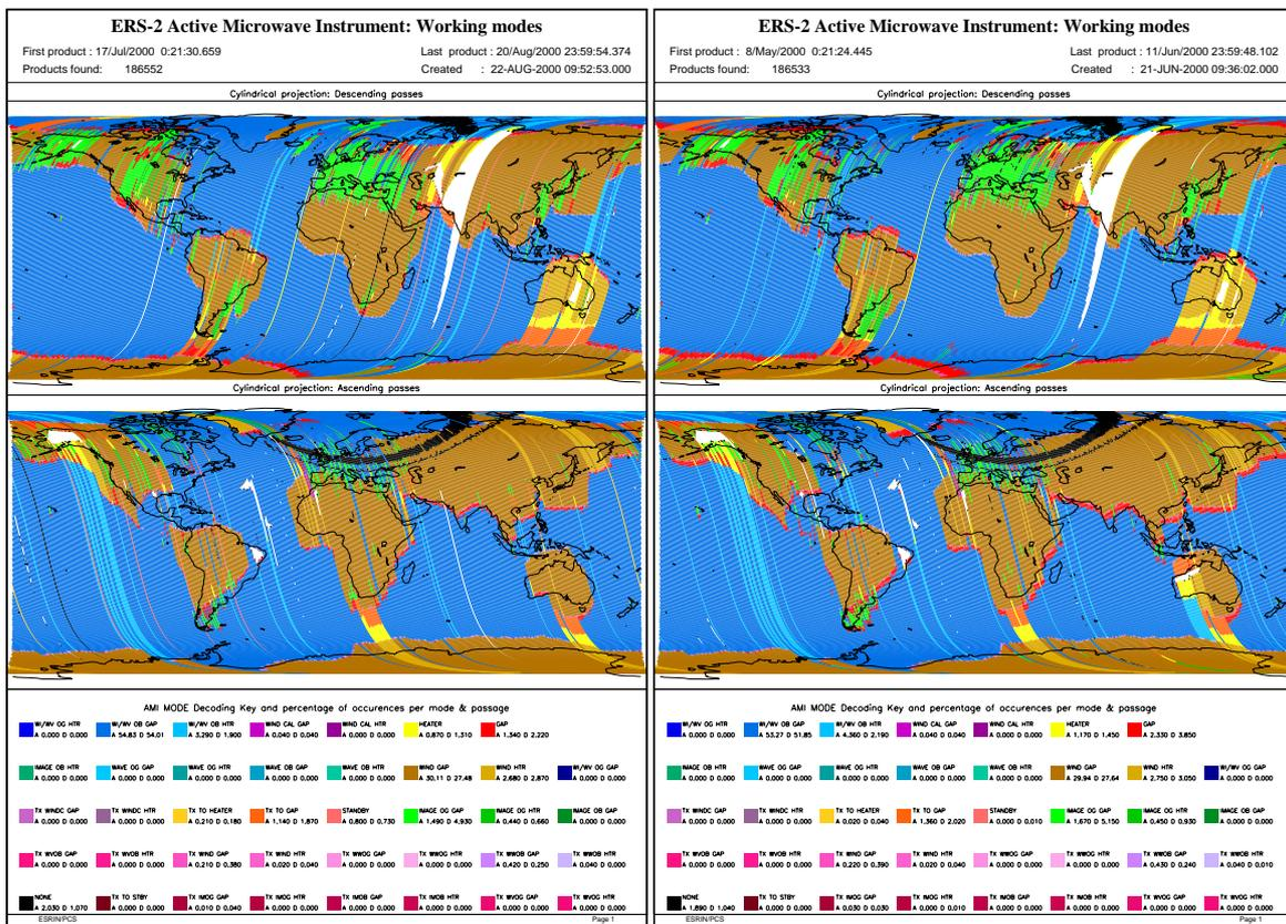
Fig. 13 ERS-2 AMI working modes. Left panel cycle 55; right panel cycle 53
