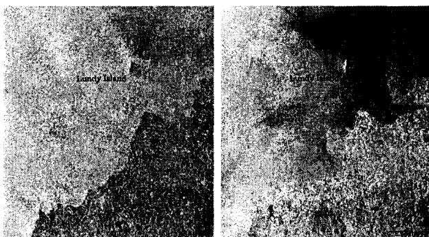
Figure 4. ERS-1(left) and ERS-2 (right) SAR images of the region extending from the southern Carmarthen Bay to the Bristol Channel on February 25 and 26, 1996, respectively. Darker filaments observed on February 26 represent lower backscatter returns associated with oil slicks reaching the Bristol Channel.
