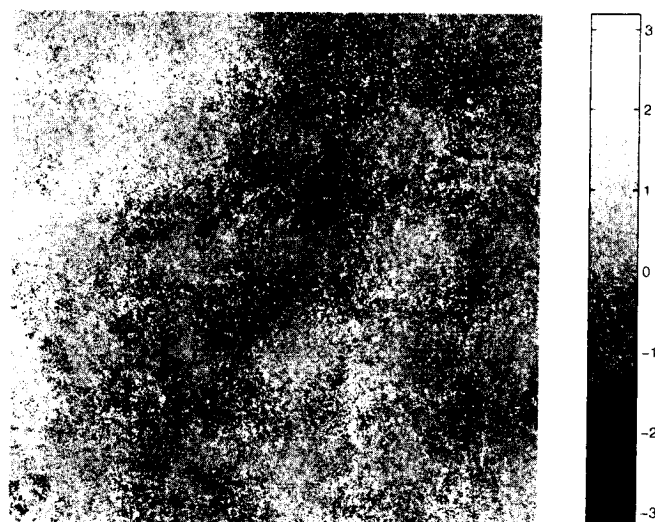
Fig. 3. The effect of a meteorological frontal zone on the interferometric phase
