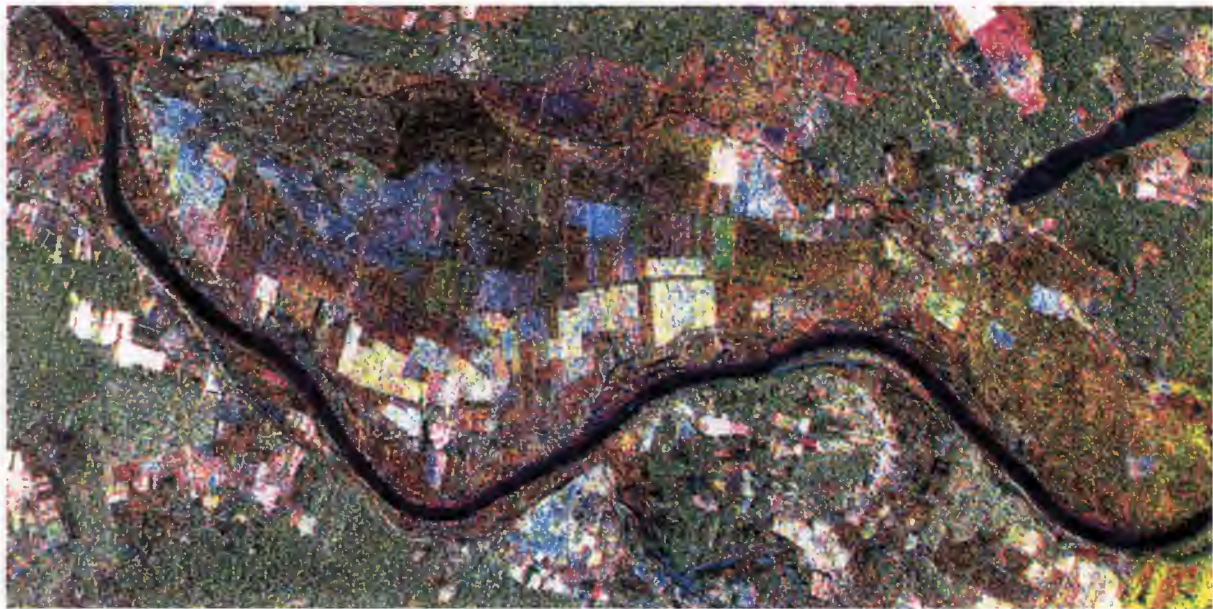
Figure 1. ERS multitemporal SAR imagery of selected test site Mödlich ( 11^{\circ}25'E and 53^{\circ}05'N ) on the River Elbe (3 * 3 filtered). Colour coding: red: 23-Mar-1996, green: 24-Apr-1996, blue: 11-Apr-1996.
