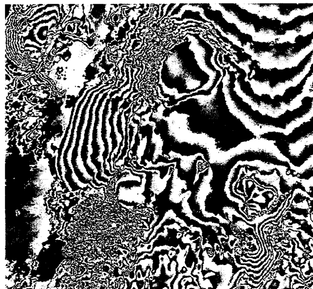
Fig. 3 ERS-1/ERS-2 tandem INSAR phase image of Vatnajökull from Dec. 30/31, 1995 with 2\pi elevation of 68 m.
