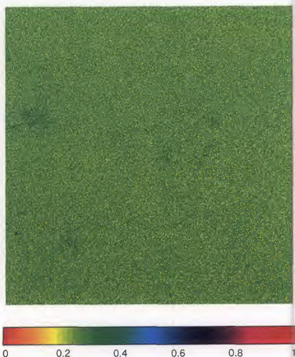
Fig. 6. Coherence image after a 3.5 year time interval, using 2 \times 11 independent samples for the coherence estimation
