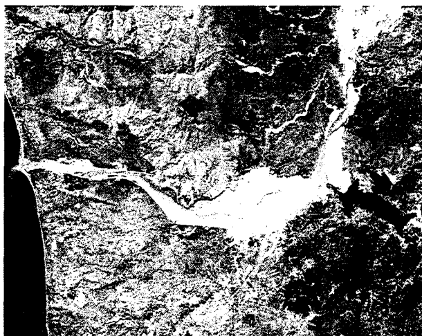
Figure 4A. Santo Tomas Basin. February 12, 1995 SPOT-P image. The high level of the stream flow, manifested by darker tone along the main active channel, has emphasized the distinct boundary of the existing high lahar terraces, in white color.
