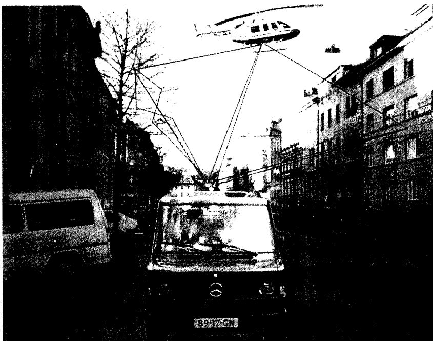
Fig.1: Test run of ESTEC's Land Mobile L- and S-Band Beacon Terminal (LMBT) in the city of Graz (Conrad-von-Hötzendorf-Strasse). The space segment is simulated by a slowly flying helicopter carrying L- and S-band beacon transmitters. Received signals are recorded and analysed with respect to shadowing (blockage) and reflection (multipath propagation), and their correlation with type of environment.
