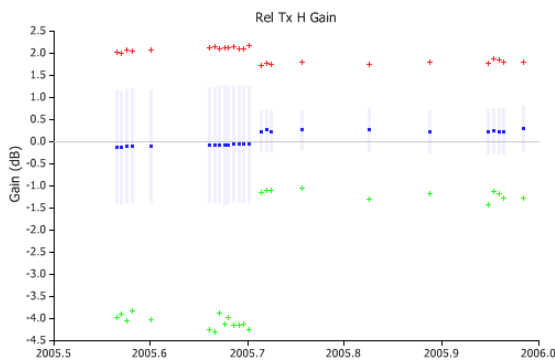
Figure 5(a). ASAR TRM Antenna Gain before and after the ASAR Antenna Reset#1 (Tx H Gain only)
