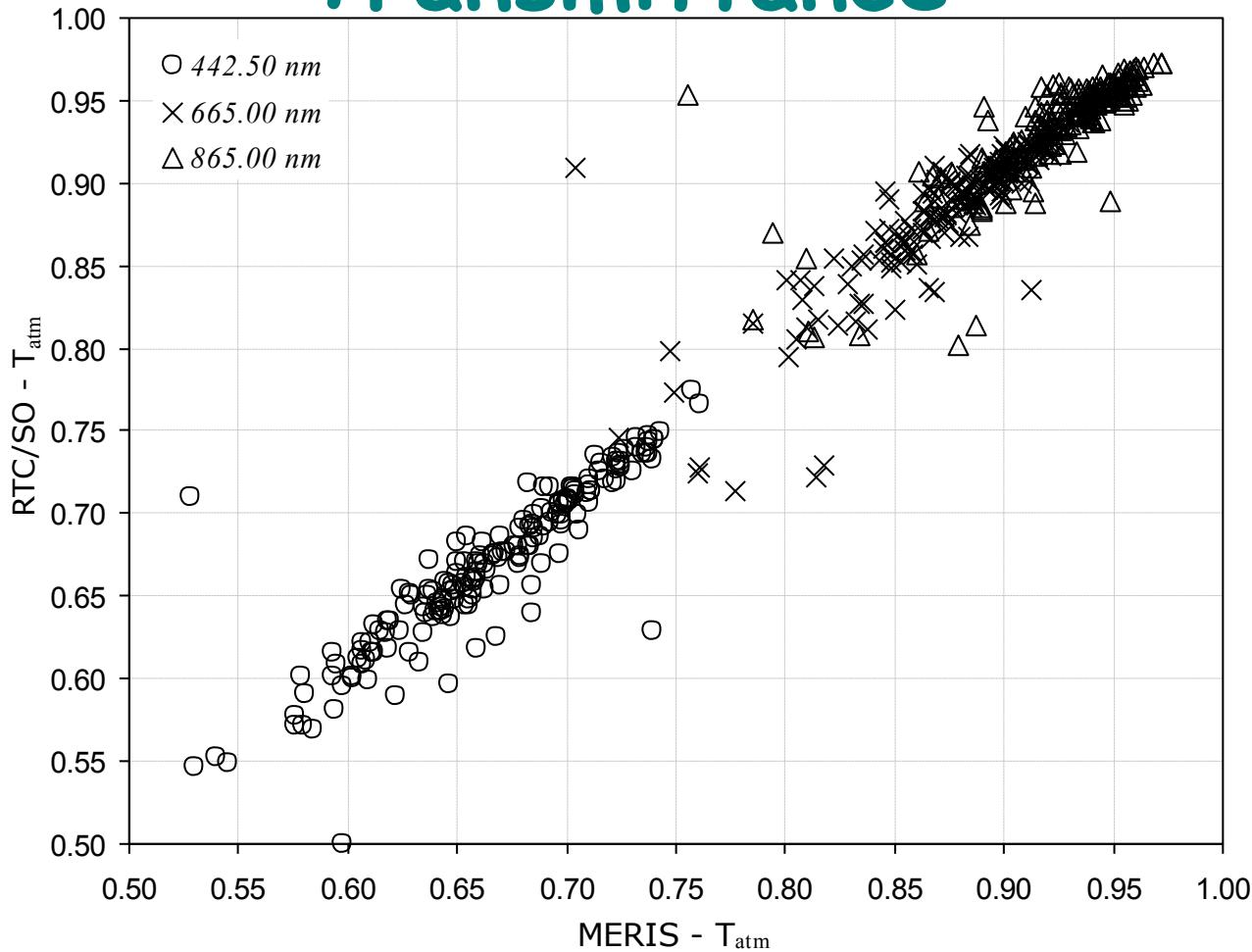
Atmospheric transmittances ( $T_{atm}$ ) in  $B_{02}$  (442.5 nm),  $B_{07}$  (665 nm) and  $B_{13}$  (865 nm).
