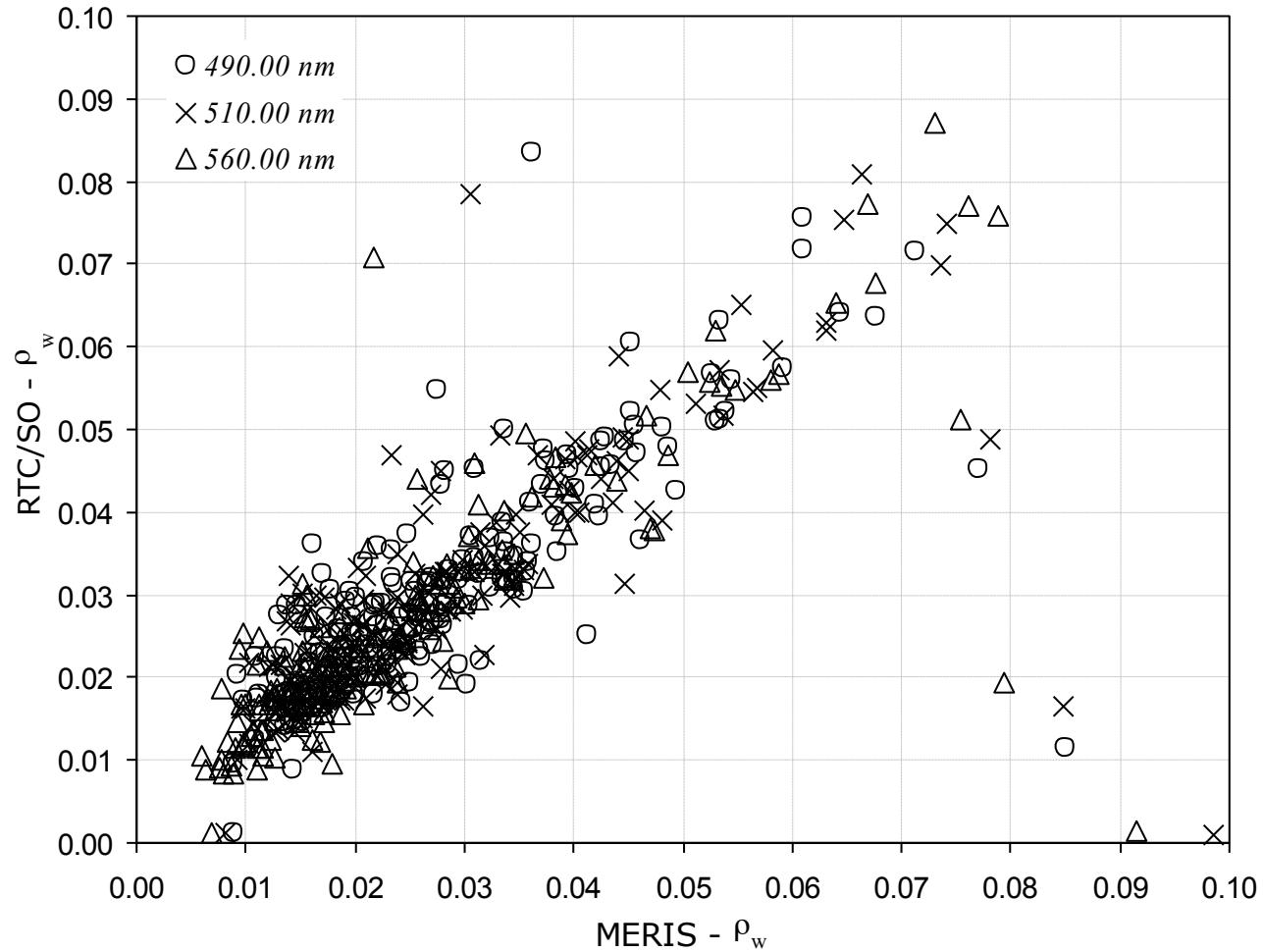
Marine reflectances ( $\rho_w$ ) in  $B_{03}$  (490 nm),  $B_{04}$  (510 nm) and  $B_{05}$  (560 nm).
