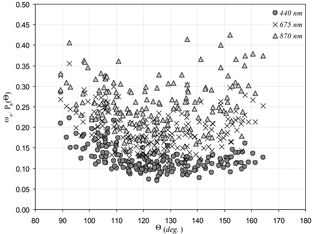
*Aerosol phase function times single scattering albedo,  $\omega_0(\lambda)P_a(\Theta,\lambda)$*
