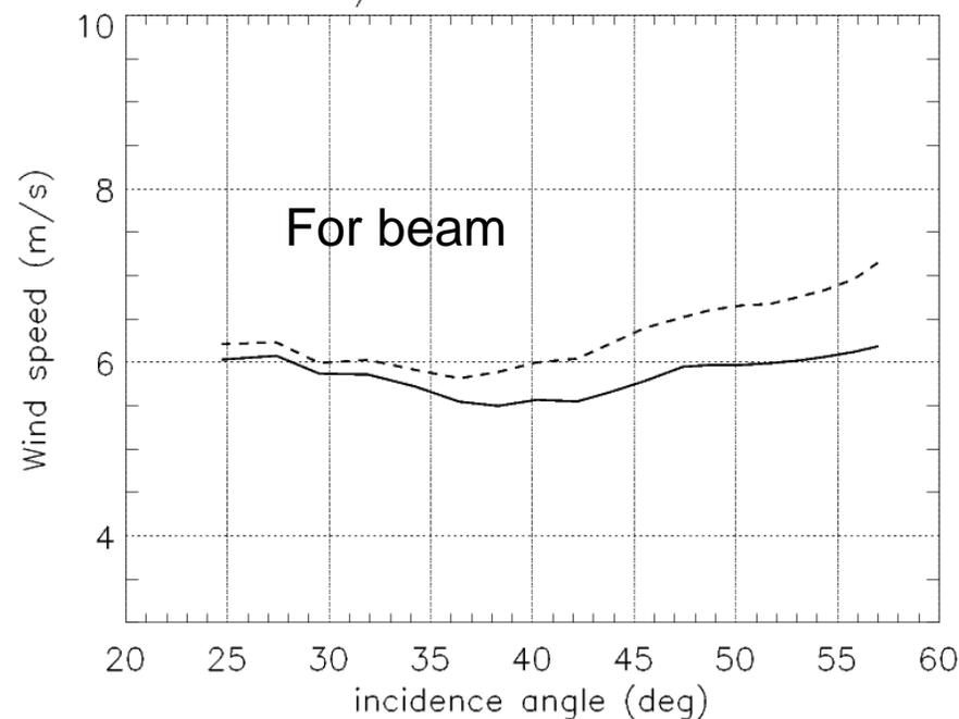
**Impact of noise subtraction increase with increasing incidence angle (decreasing sigma)**
