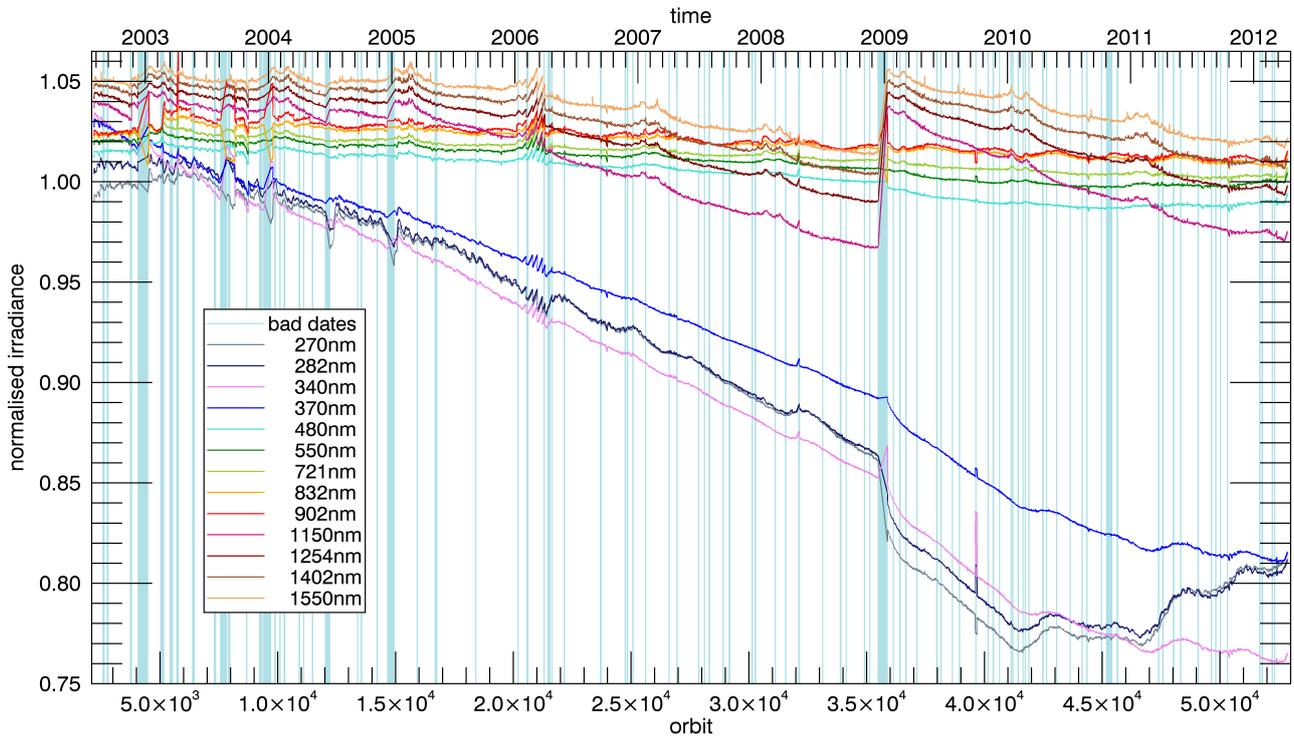
Figure 5: SCIAMACHY SSI time series of Version 7; normalised to solar spectrum of 27.02.2003 shown in Fig. 3
