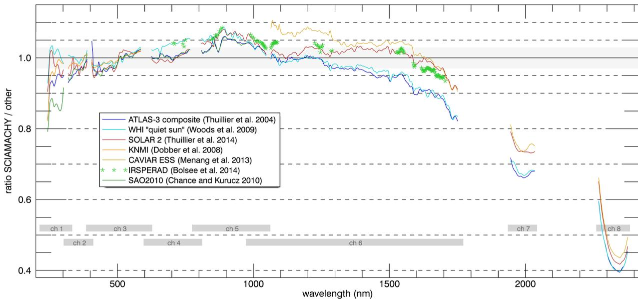
Figure 8: Ratio of SCIAMACHY to solar reference spectra shown in Figure 7, convolved to resolution of 10 nm.
