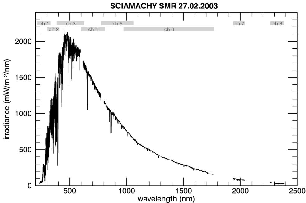
Figure 2: SCIAMACHY solar mean reference spectrum (SMR) data version 8 for 27 February 2003, provided for Sun-Earth distance of 1 AU; SCIAMACHY spectral channels are indicated
