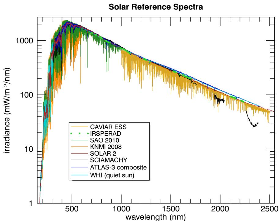
Figure 7: Solar reference spectra in comparison to the SCIAMACHY solar reference spectrum (27.02.2003)
