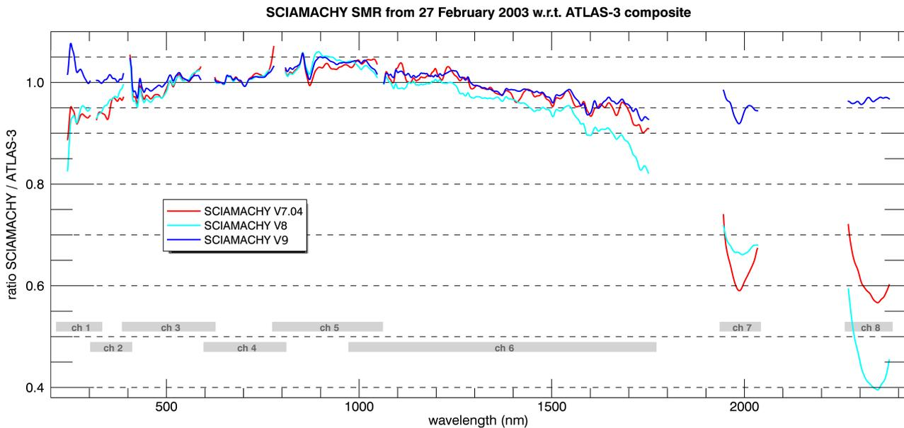
Figure 3: SCIAMACHY SSI of 27 February 2003 in different data versions in comparison with the ATLAS-3 composite. All spectra are convolved with a 10 nm Gaussian before generating the ratio.
