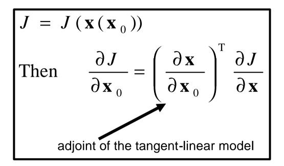
Transpose reverses the sequence of matrices in the chain rule, so the tangent linear model is run BACKWARDS in time.
