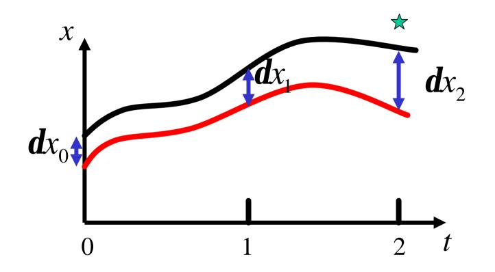
$$\begin{aligned} x_{1} &= M(x_{0}) \\ dx_{1} &= \frac{\partial M}{\partial x} \Big|_{x_{0}} dx_{0} \end{aligned} dx_{2} &= \frac{\partial M}{\partial x} \Big|_{x_{1}} \frac{\partial M}{\partial x} \Big|_{x_{0}} dx_{0} \end{aligned}$$
