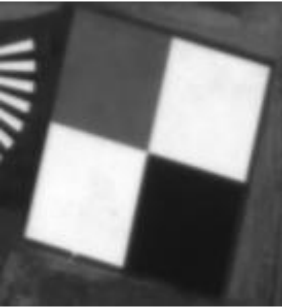
Edge Detection (Across, 12.20 deg, Fit Err:1.7)
