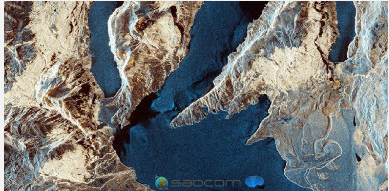
Detail of the first SAOCOM-1A image: StripMap (DS5), Dual Pol (DV) Composed image (R: VH, G: 2VH + VV, B: VV)
