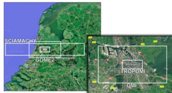
Figure 1: This figure demonstrates the satellite footprint size comparison between GOME-2/MetOp and SSP/TROPOMI.
