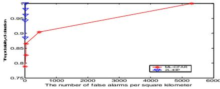
Figure 11: Probability of detection vs. false alarm rate of ML-CFAR and 2L-IHP
