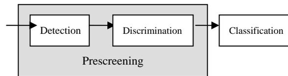
Figure 1: Flowchart for ATR system
