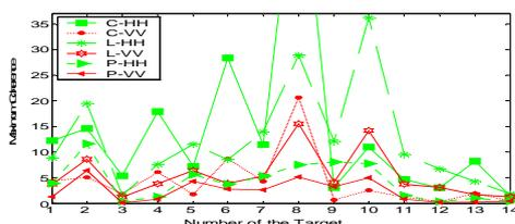
Figure 15: Coherence of 14 man-made targets in HH/VV SAR images
