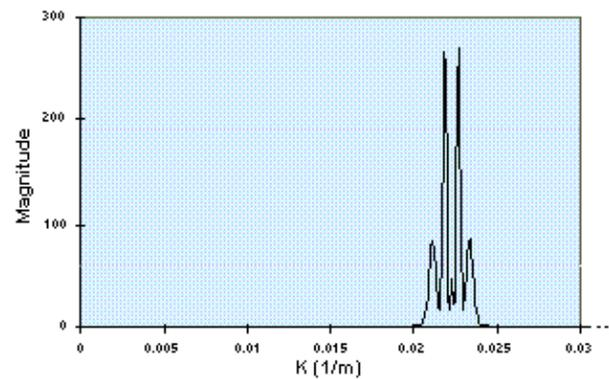
Fig. 7: Power spectrum corresponding to a terrain modelled by  $y = c \cdot \exp[-(x-m)/2s^2]$ , with  $c=500$ ,  $m=334012$ ,  $s=137471$ ,  $x_{max}=374425.44$ ,  $x_{min}=293599.20$ ,  $b=100$ ,  $q_0=90$ .
