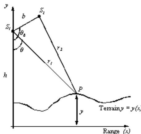
Fig.1: Typical geometry of a cross-track interferometric SAR
