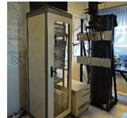
Figure 11: Thessaloniki lidar system (THELISYS)
