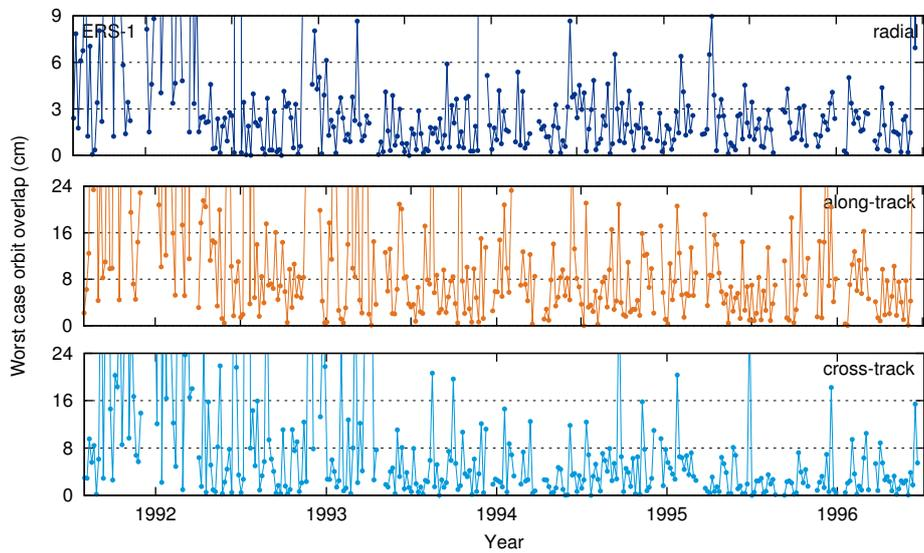
Figure 2.8: Worst case orbit overlap in centimetres for ERS-1 DEOS solution.
