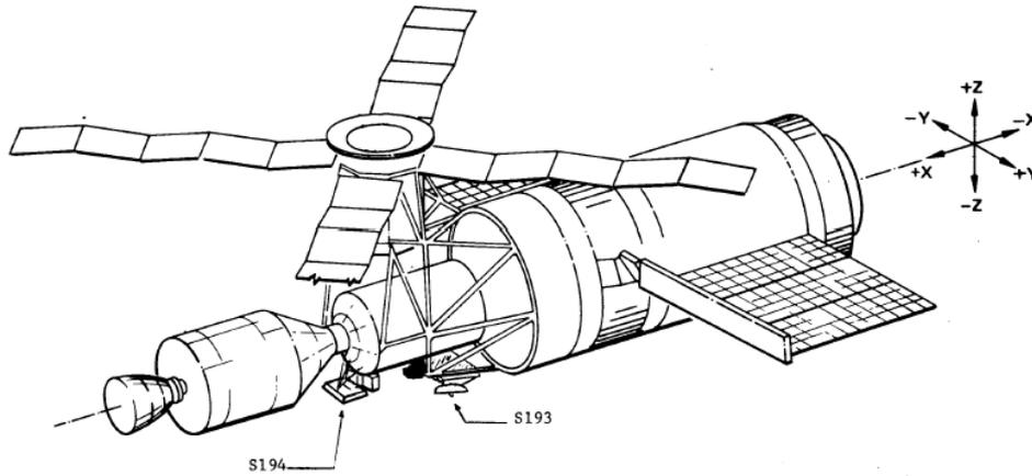
Fig. 1 - Location of radiometers on Skylab
