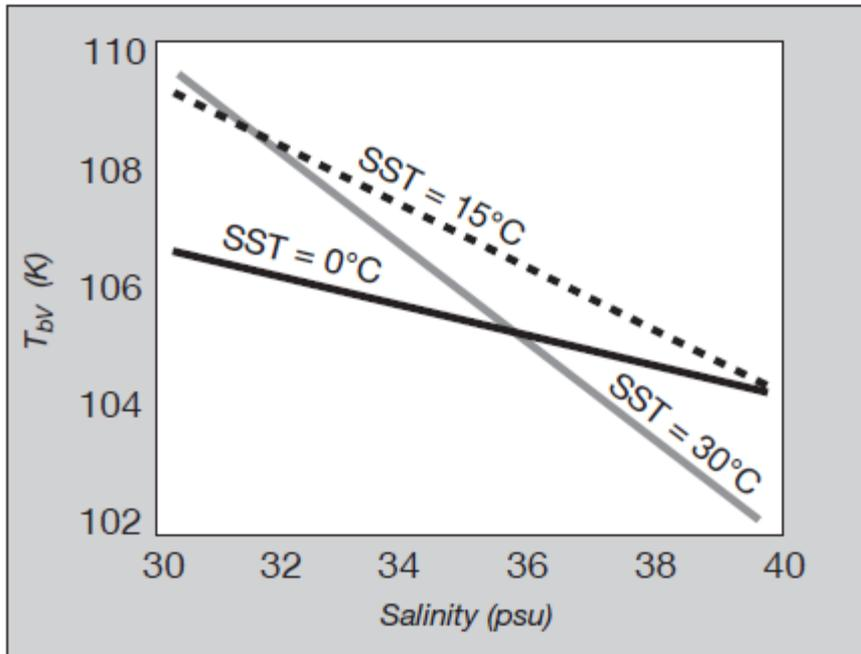
The sensitivity of the brightness temperature at L-band to SSS remains small. It depends on the sea surface temperature (SST):
