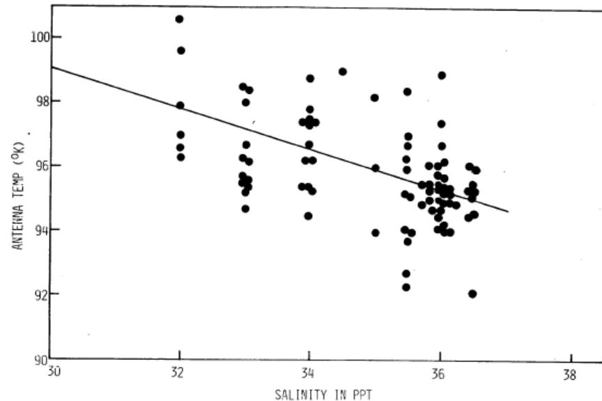
Fig. 17 - Antenna temperature dependence on salinity
