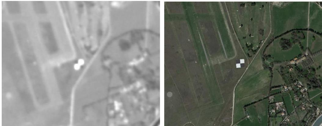
Figure 4-4: Salon-de-Provence MTF target as captured on the 07 April 2021 shown using the 5m resolution panchromatic band (left) and as shown using Google Earth (right) for the same geographical extent.
