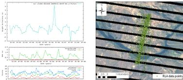
To calculate discharge (Q in m<sup>3</sup>/s) from altimetry at these points, empirical equations derived from Manning’s equation which need only the area (A in m<sup>2</sup>), the wetted perimeter (P in m) and the slope (S) are then used.
