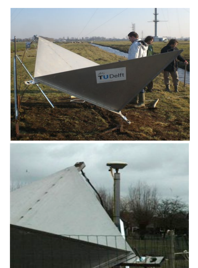
Figure 6: Corner reflectors equipped with GPS receivers (Cabauw, the Netherlands).
