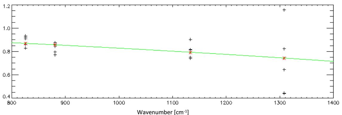
Figure 2: Modulation efficiency as deduced from combined IF16 and IF4 measurements. Black: individual values, green: second order polynomial fit, red: values for the four non-linear channels taken from the fit.
