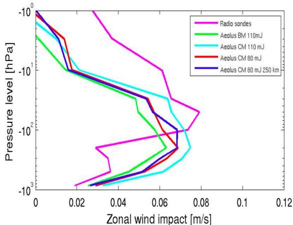
Aeolus zonal wind impact on operational weather forecasts. The impact of continuous mode is higher than burst mode. The impact is only slightly degraded when going from 110 mJ to 80 mJ laser pulse energy, or when going from 100 km to 250 km horizontal sampling.
