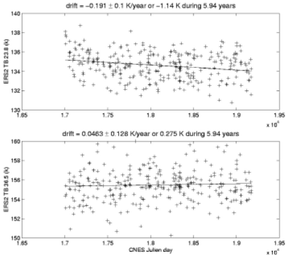
Figure 2 : Drift of the ERS2 brightness temperatures, using cross-over points between the two missions with selection of the coldest TMR 21 GHz brightness temperatures over ocean.
