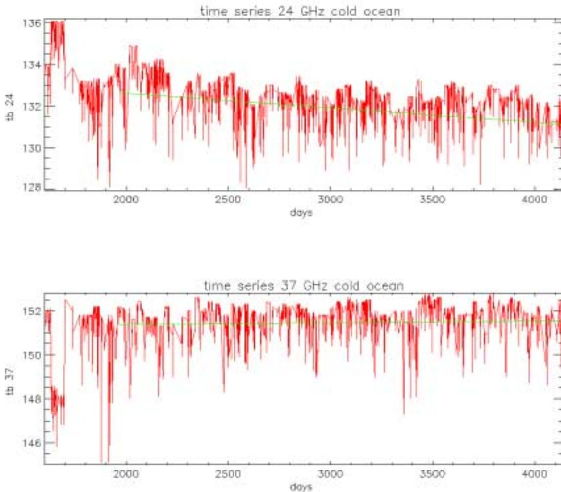
*Figure 1 : Long term monitoring of the coldest TBs over the oceans for ERS2-MWR. Mean and standard deviation of data (lower than a given threshold) were computed for each cycle, then we kept the data lower than the mean minus two times the standard deviation were kept. Dates (in days) are referenced to January 1<sup>st</sup>, 1991. TBs are in Kelvin, the two channels are labeled by their respective frequency.*
