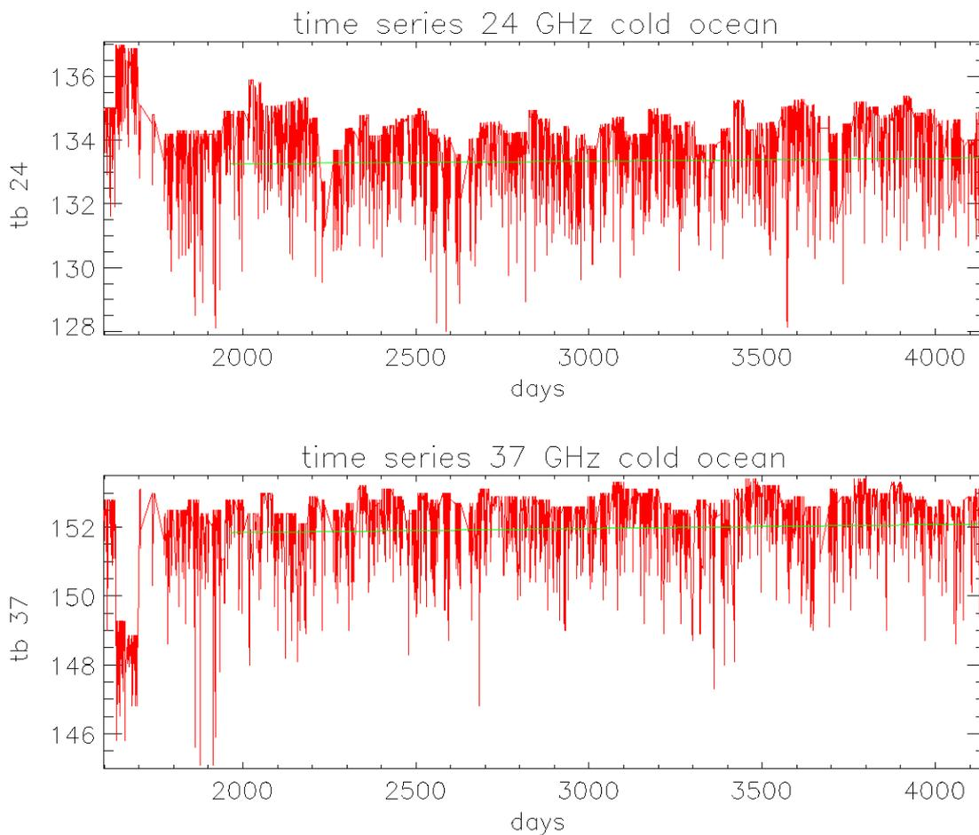
*Figure 4 : same as figure 1 after correction of the 23.8 GHz TBs drift.*
