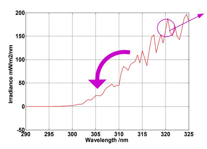
Solution: subtract an instrumentdependent fraction (%) of light at 320 nm to the count rates measured at the 5 operating wavelengths in the UV range
