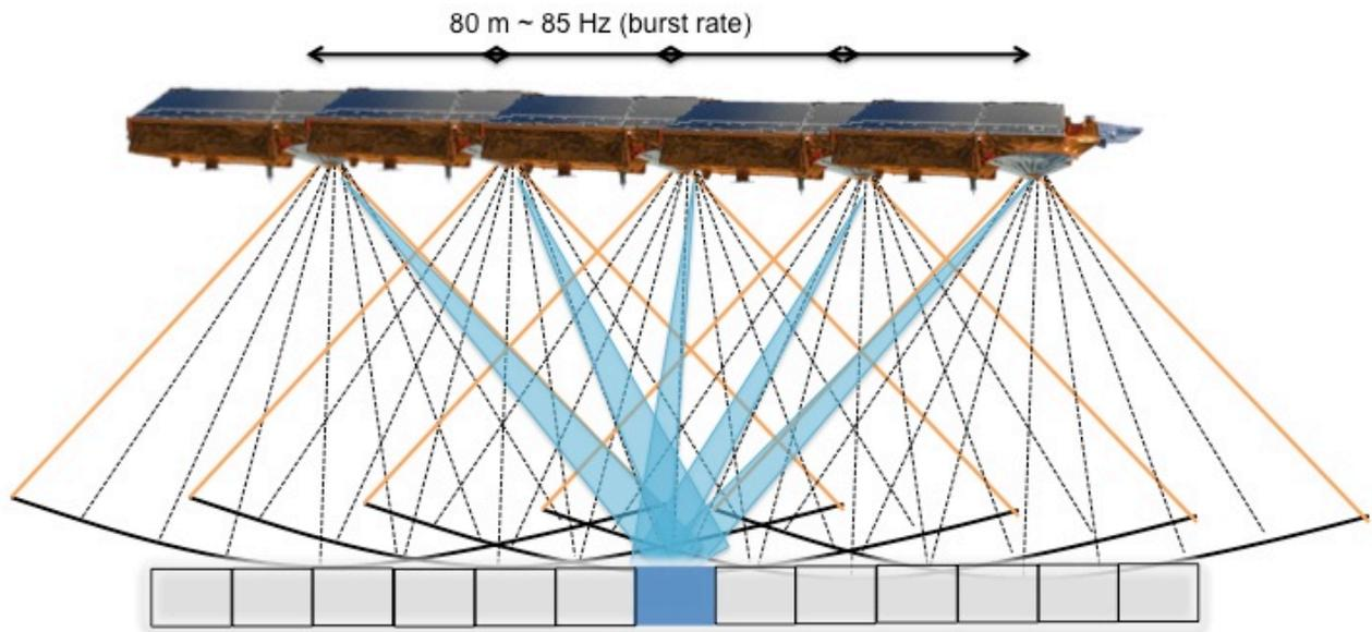
Figure 3: Geometry of multi-looking
