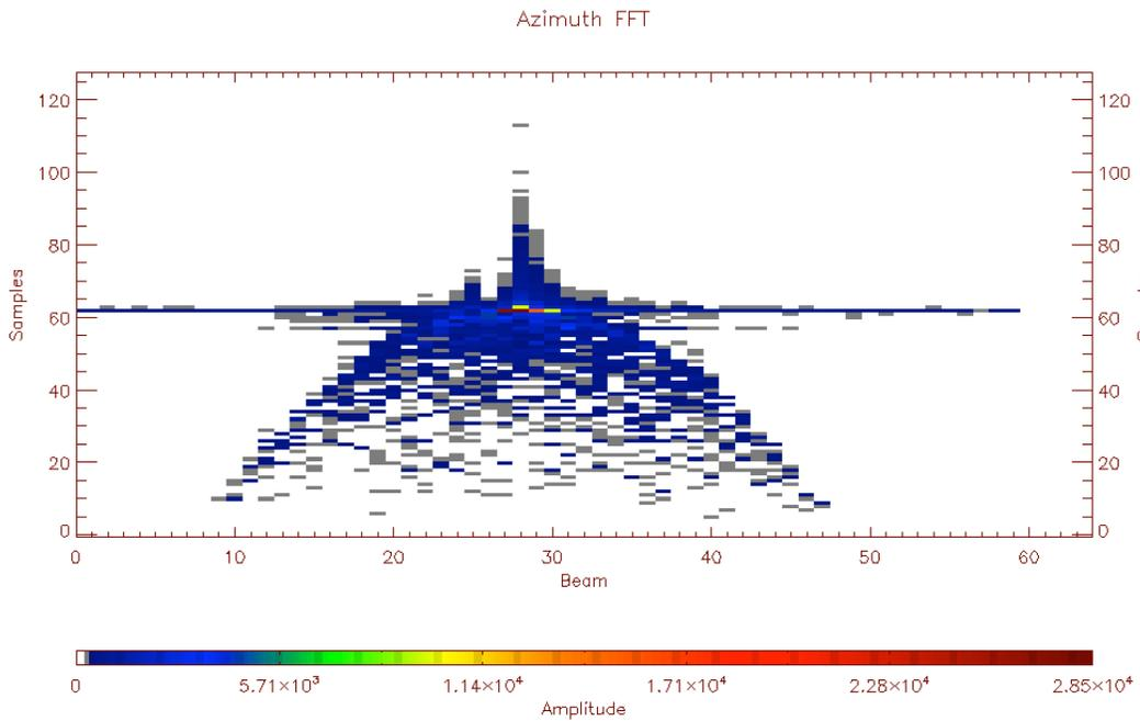
**Figure 12: Azimuth FFT of a single burst: the nadir clutter is the 'line' in the middle**
