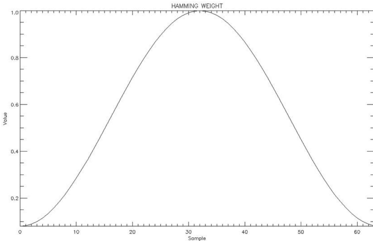
**Figure 11: Hamming weighting function**
