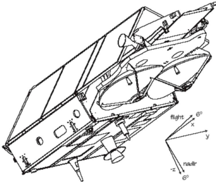
**Figure 6: Satellite Reference Frame**
