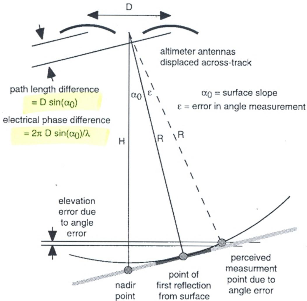
Figure 4: SARin mode across-track angle determination
