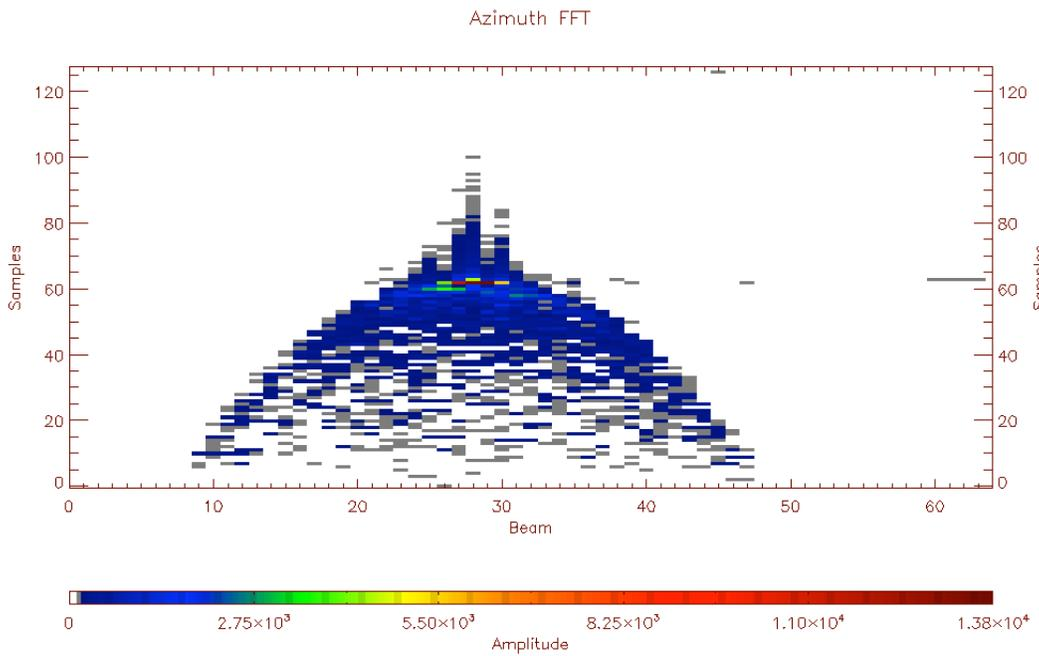
**Figure 13: Azimuth FFT of a single burst with hamming: the nadir clutter is reduced**
