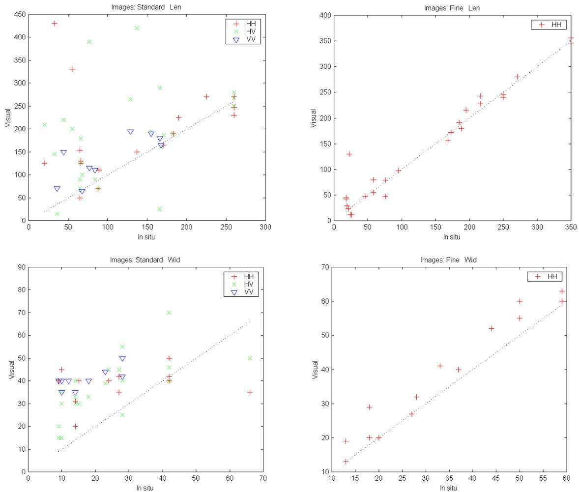
Fig. 2. Comparing visually estimated vessel size to real vessel size. Top row: Length (m). Bottom row: Width (m). Left column: Standard resolution, i.e. 25 m multi-look (ERS-2, ASAR Image and Alternate polarisation and RADARSAT Standard). Right column: Fine resolution, i.e. 8 m single-look (RADARSAT Fine). Symbol shape and colour indicate polarisation.
