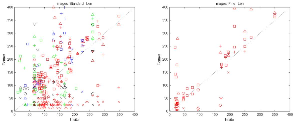
Fig. 3. Vessel length as estimated by the various ship classification algorithms from Table 1 against real length. Left for 25 m multi-look images, right for 8 m single-look images. In this figure symbol shape signifies the algorithm and colour signifies polarisation (HH = red, HV = green, VV = blue, and a composite result from two polarimetric channels = black).
