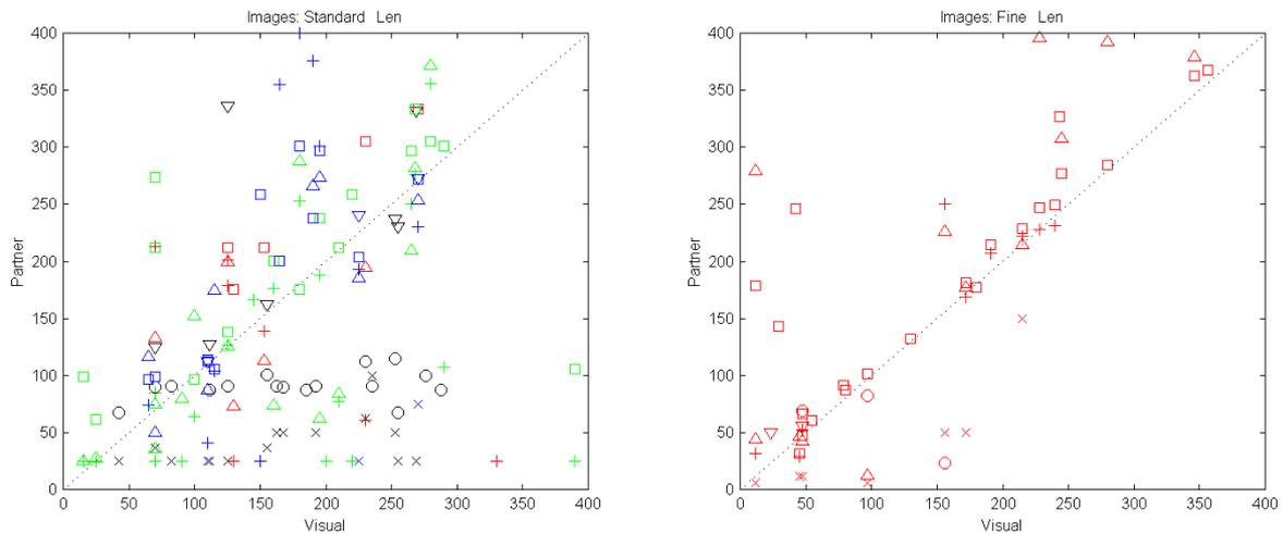
Fig. 4. Comparing automatic systems vessel length estimates to visual length estimates. Legend as in Fig. 3.
