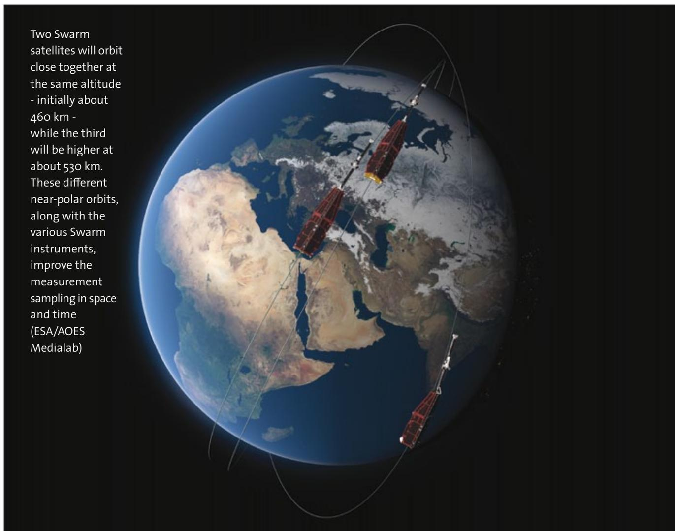
Two Swarm satellites will orbit close together at the same altitude - initially about 460 km - while the third will be higher at about 530 km. These different near-polar orbits, along with the various Swarm instruments, improve the measurement sampling in space and time (ESA/AOES Medialab)
