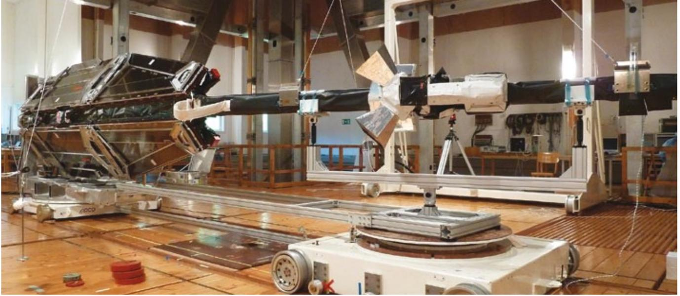
↑ One of the Swarm satellites, with boom deployed, undergoing tests at IABG's Magnetic Field Simulation Facility in Ottobrunn, Germany. The tests are carried out in a magnetically clean environment – hence the wooden floor (ESA/IABG)
